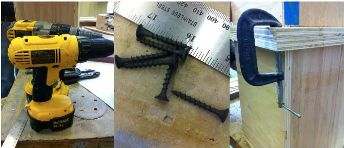
Figure 18. Material used to fixing the wood box together
