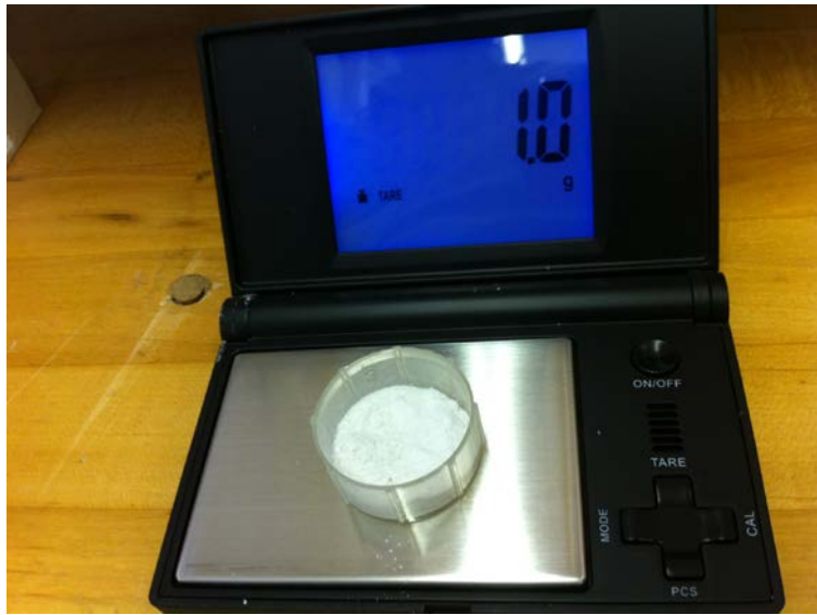
Figure 32. Weigh 1.0 g powder – Sona 2007 Scale accuracy \pm 0.05 grams
