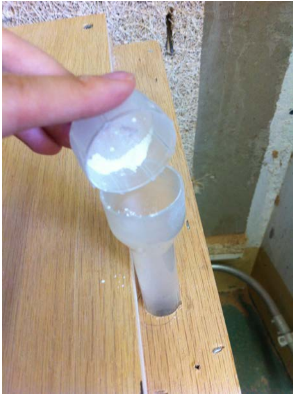
Figure 33. Using the powder tunnel to place the material
