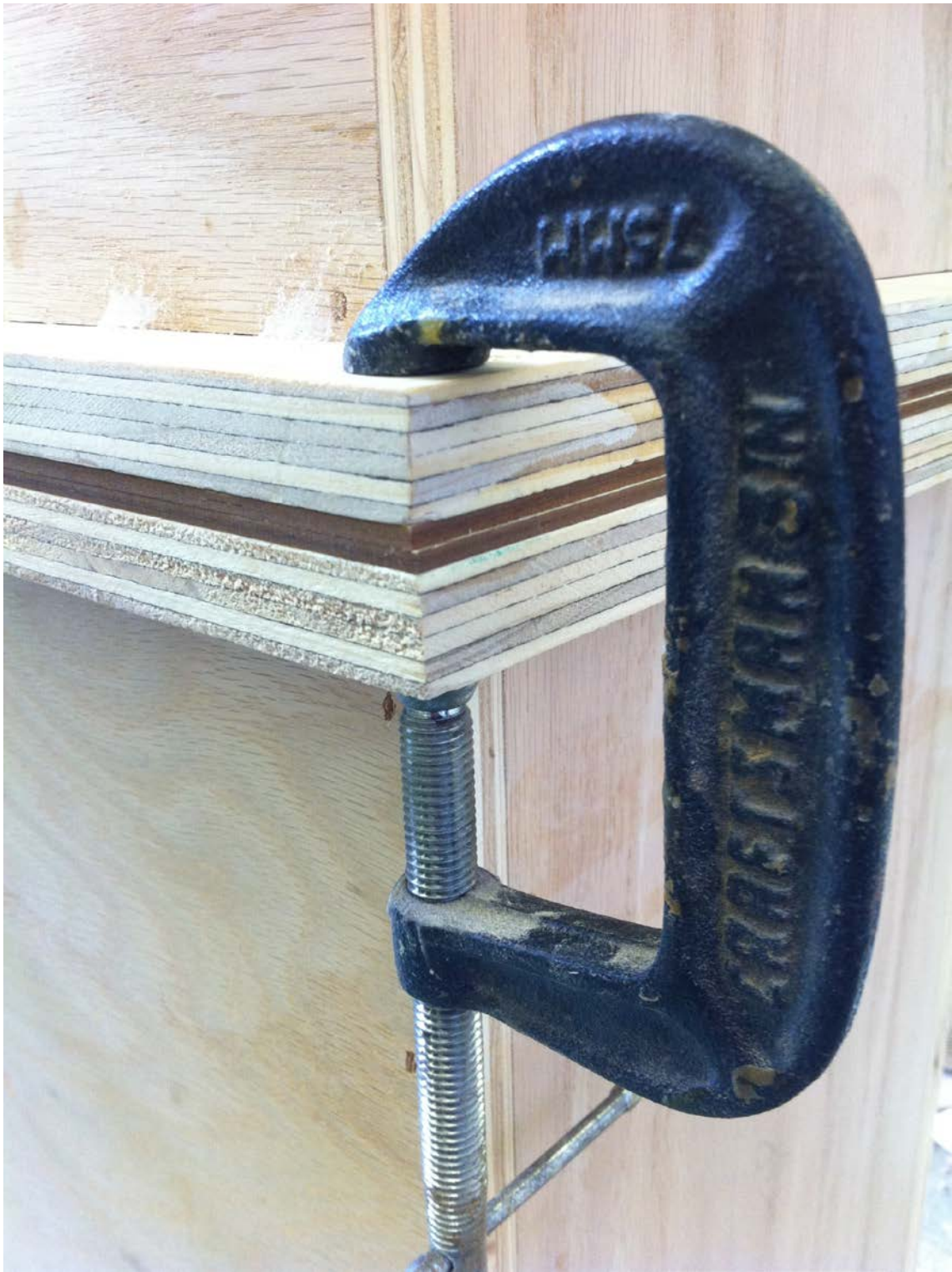
Figure 28. C-clamp in place to hold the chambers still
