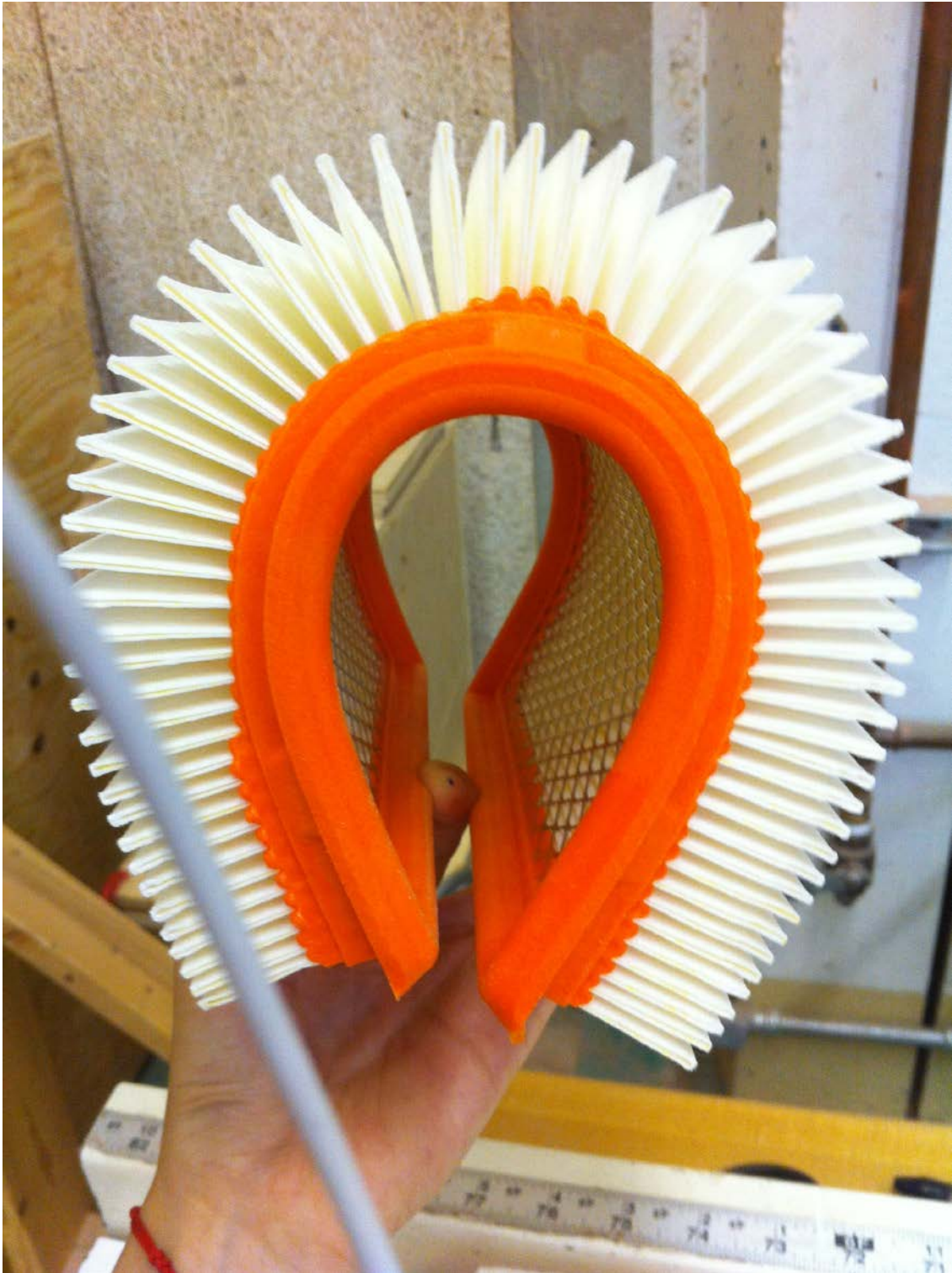
Figure 27. Air filter shown in a flexed position
