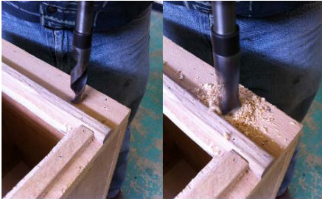
Figure 17. Drill a hole to fit the funnel on the top of box
