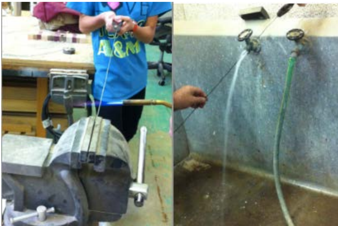
Figure 14. Straightening the iron wire and cool it down
