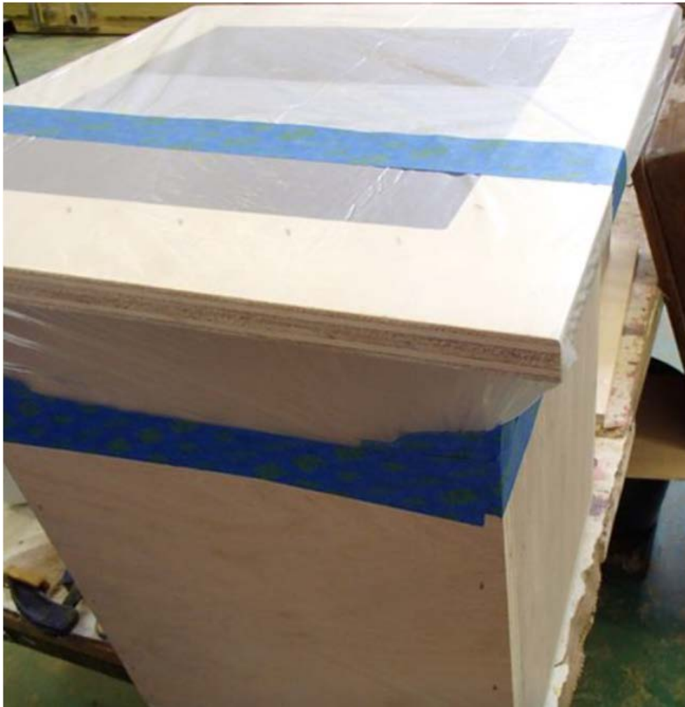
Figure 5. Taped and sealed plastic sheeting
