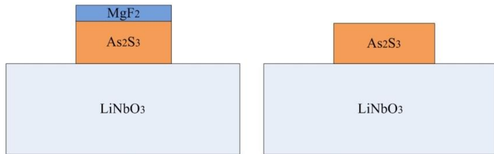
Figure 3.1 (a) \text{As}_2\text{S}_3 waveguide with \text{MgF}_2 cladding; (b) without cladding
