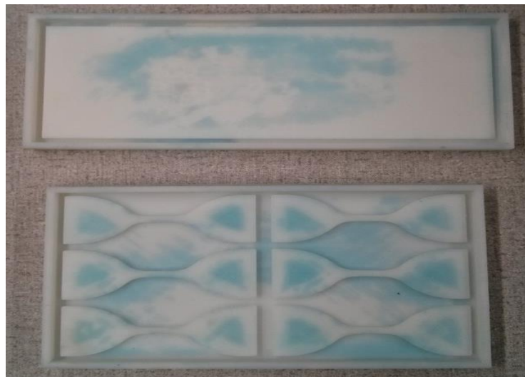
Figure 18. Tensile specimen and planar specimen ABS molds
