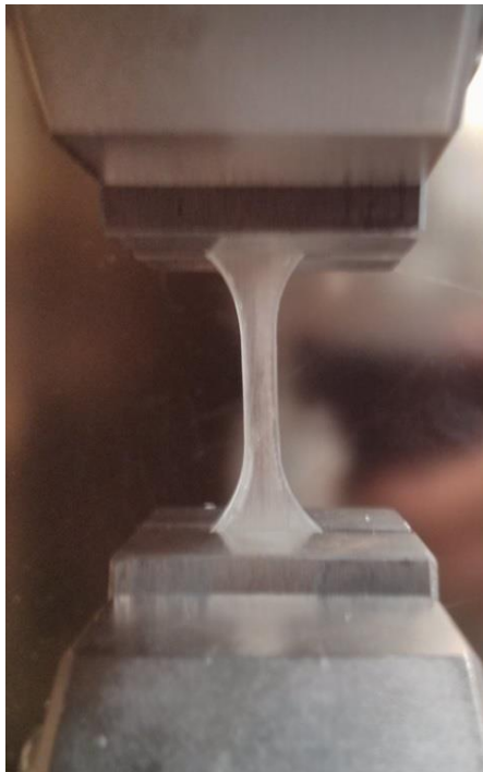
Figure 26. Tensile test specimen was positioned between top and bottom grips.
