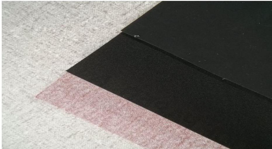
Figure 19. From the front to the back 150,320,600 grit sanding papers can be seen.
