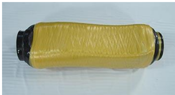
Figure 4. Reusable mandrel covered by filament. [30]
