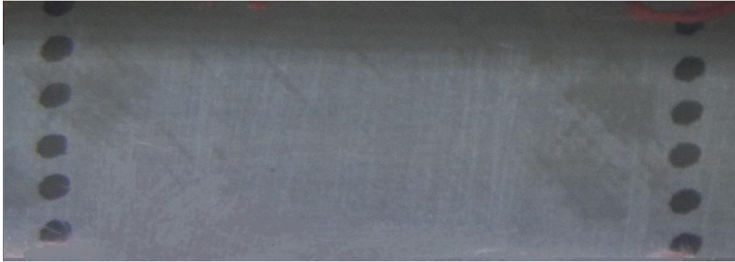
Figure 39. Black dots are marked to calculate strain for planar tension test.
