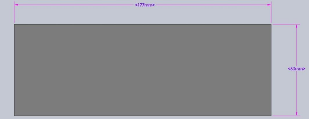
Figure 16. Planar tension specimen dimensions
