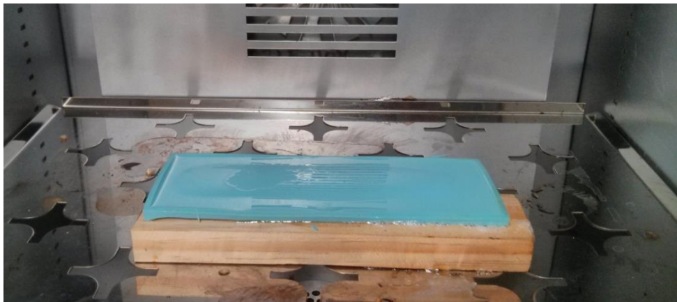
Figure 24. This picture was taken during the planar tension specimen curing process.
