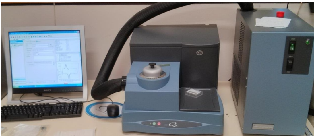
Figure 25. Test parameters are arranged by computer. Heat flow provided by right side machine. Nitrogen bottle also include in DSC whole step up.
