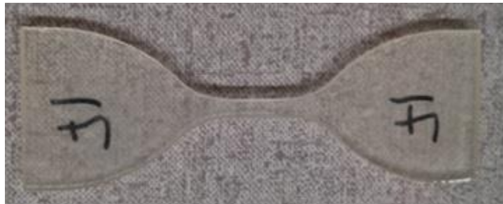
Figure 30. Dog bone tensile specimen made from epoxy-based SMP shows no visible bubbles and other flaws.
