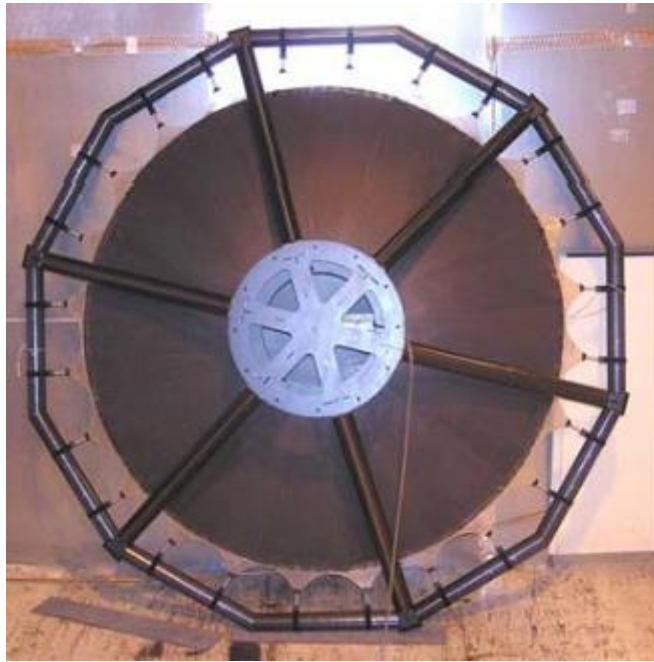
Figure 6. SMP composite reflector in the hybrid inflatable antenna. [35]
