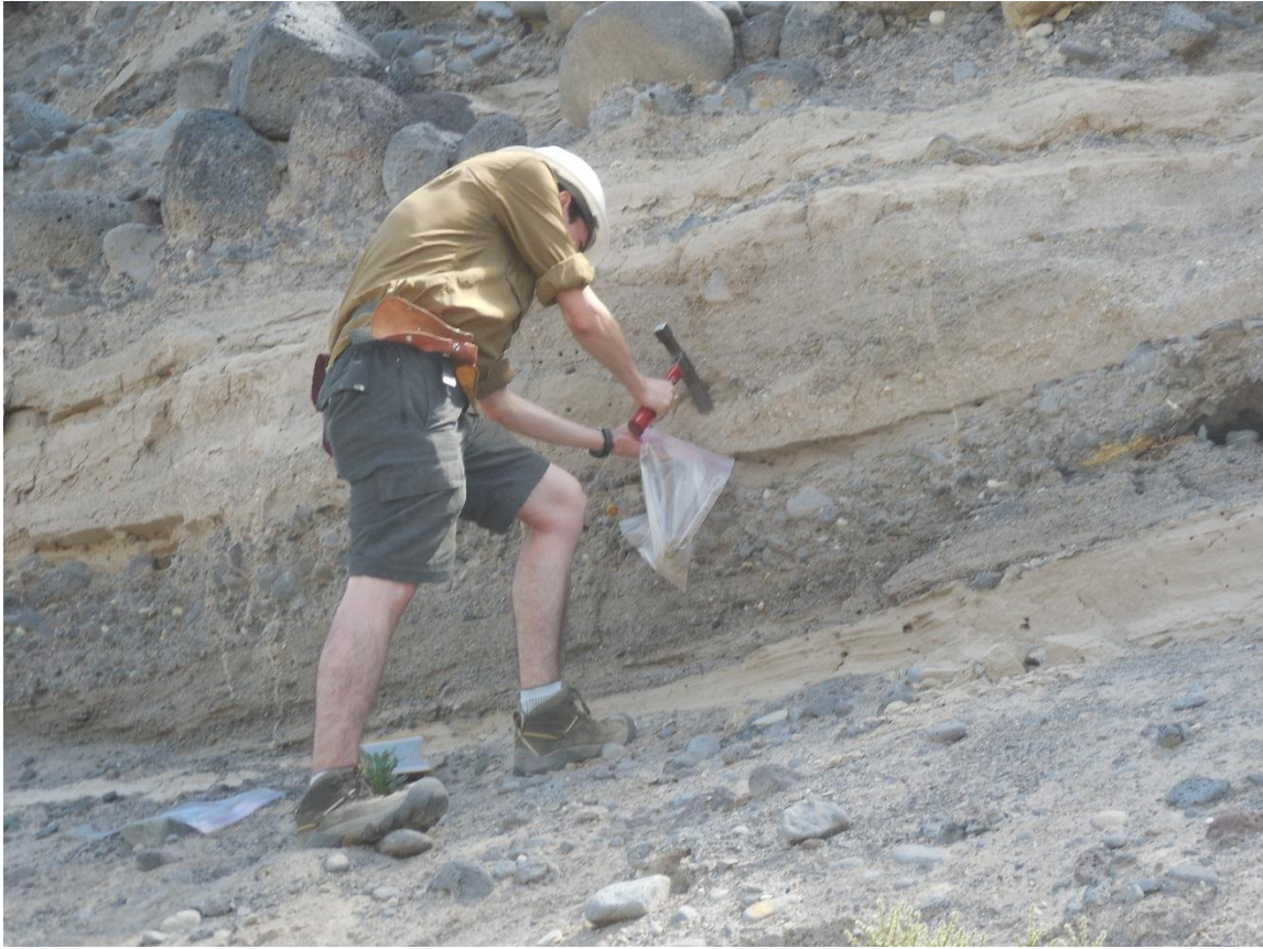
Figure 4. Sample collection using a rock hammer and collection bag.
