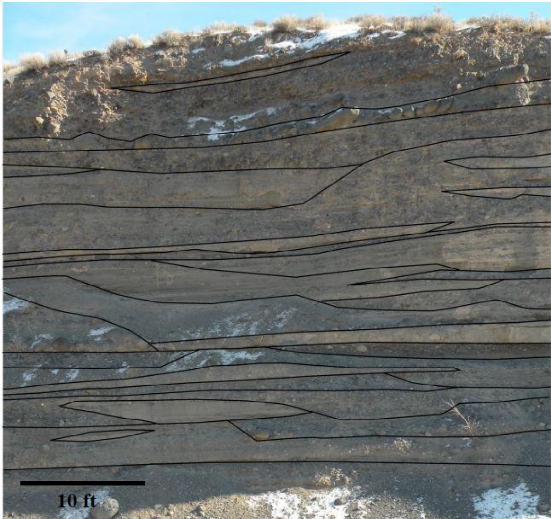
Figure 40. Example of lateral discontinuity of beds. Adapted from Brunk (2010)
