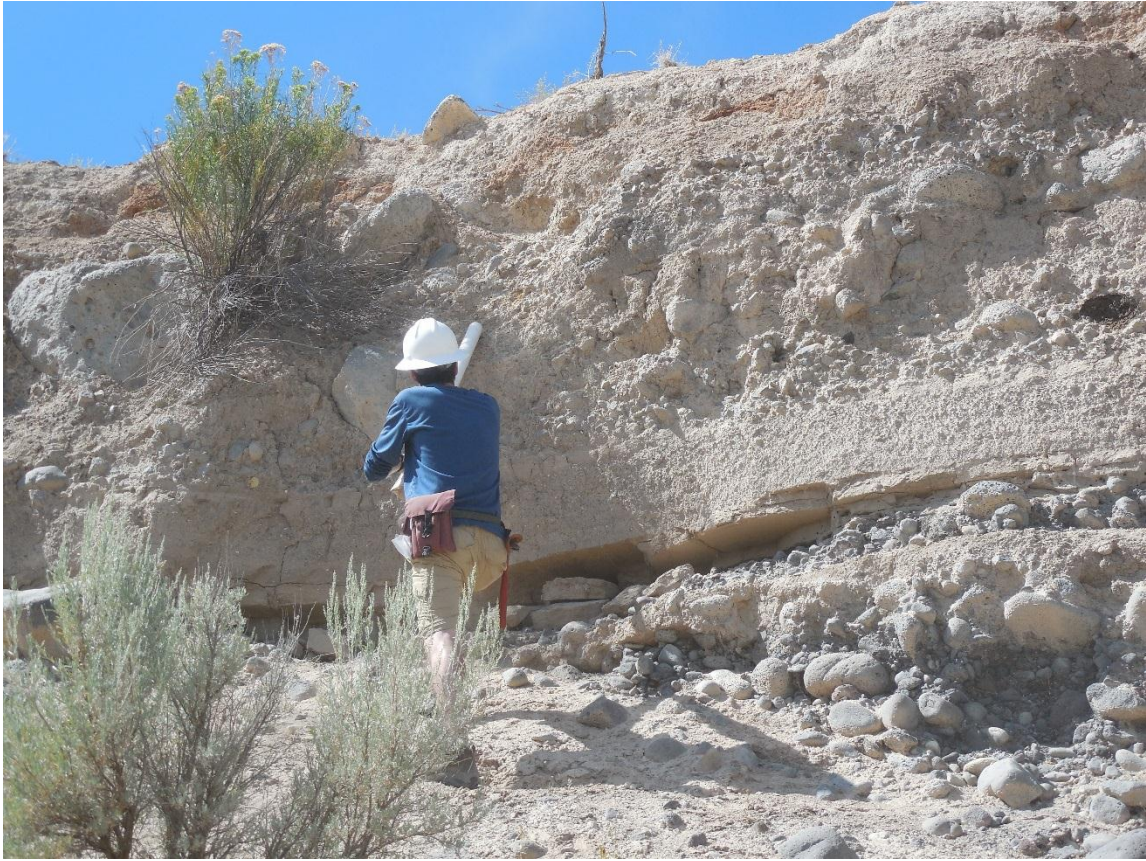
Figure 5. Sample collection using PVC collection pipe.
