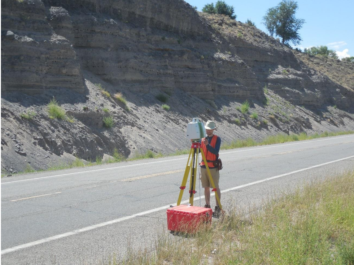
Figure 6. LiDAR scan station in use.
