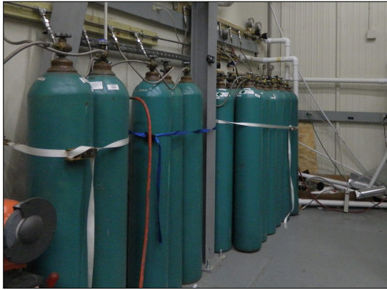
(a) Helium gas bottles hooked up to all three lines (each row of bottles makes up a line, with lines 2 and 3 running parallel to each other).
