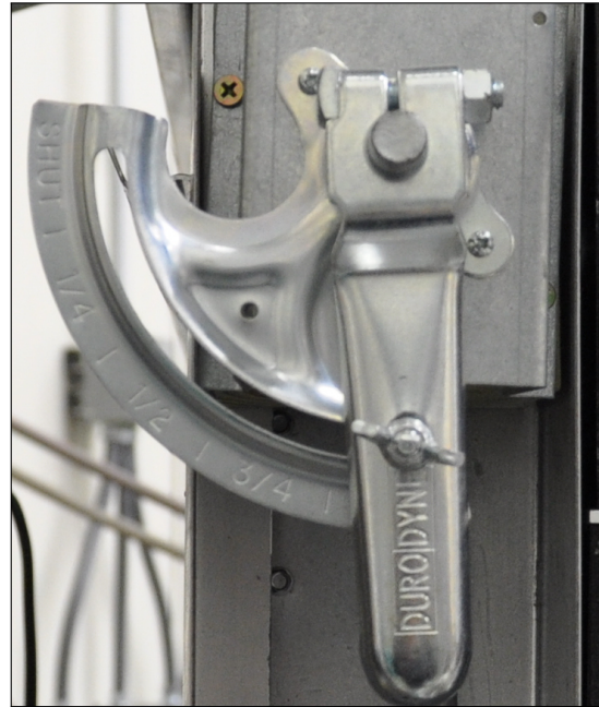
(b) Louver adjustment control arm used to manipulate the flow velocity through a given sub-layer.
