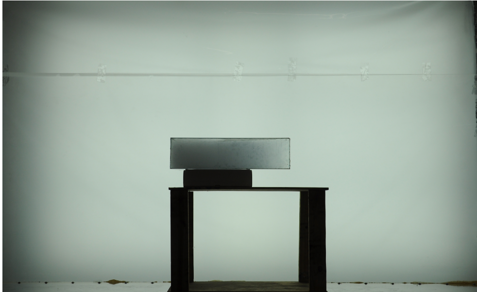
Figure 2.6: Triangular prism inside test section used for calibration of concentration curves with backlight. Image taken using Nikon ® D90 ™ camera. Fog concentration increases linearly from right to left inside the prism.
