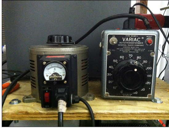
Figure 2.8: Variable transformers used for controlling internal fans in the fog splitting system. The voltage controls the fan power, and the seeding for the given stream during PIV experiments.
