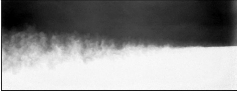
(a) Corrected instantaneous experimental image for Atwood number 0.055 with \Delta U = 0.16 \text{ m/s} . The characteristic Rayleigh–Taylor plume structures are clearly visible.
