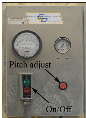
Figure 2.5: Power box used to operate fan and blade angles. The large white dial displays the pitch angle of the blades, which ensures consistency between experiments.
