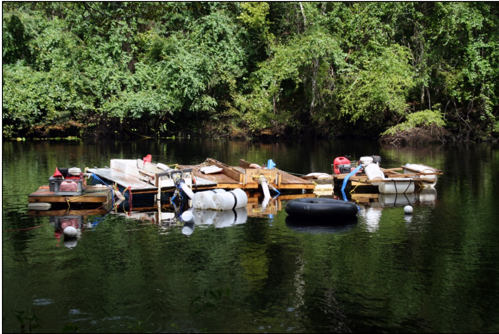
Fig. 6.1. Dredge screen setup.
