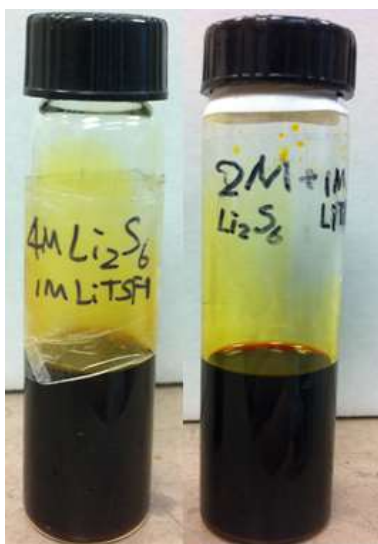
Figure 5.1 Photograph of polysulfides catholyte ( \text{Li}_2\text{S}_6 dissolved in electrolyte)
