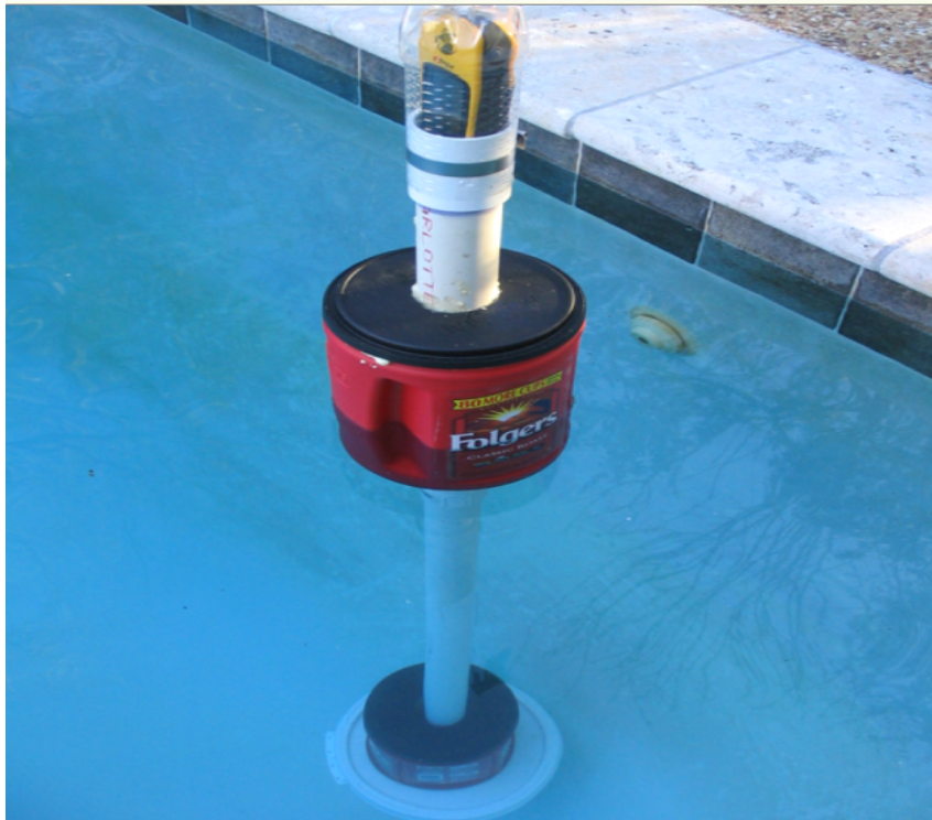
Figure 5. Prototype surface drifter used in sampling surface current in Ibaka bay (December 2012). Garmin RINO 120 series GPS is housed in the white plastic seal on top (Courtesy: Dr. Brooks)
