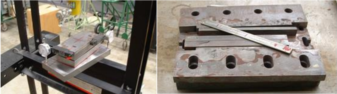
Figure 34: Spring Test Setup and Heat Treatment Fixture
