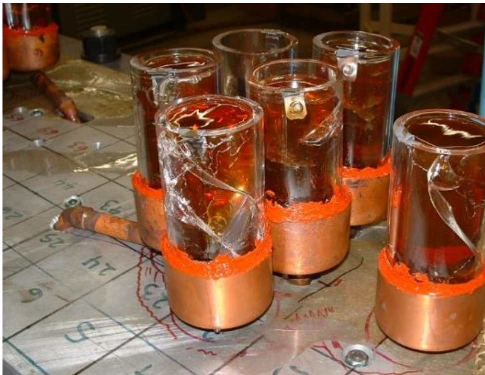
Figure 52: Cured Epoxy in Filling Cups
