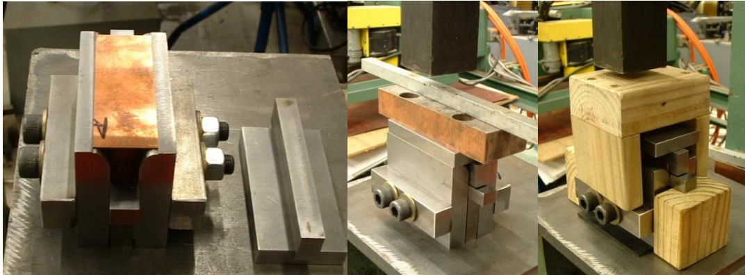
Figure 107: Copper Can Former Operation
