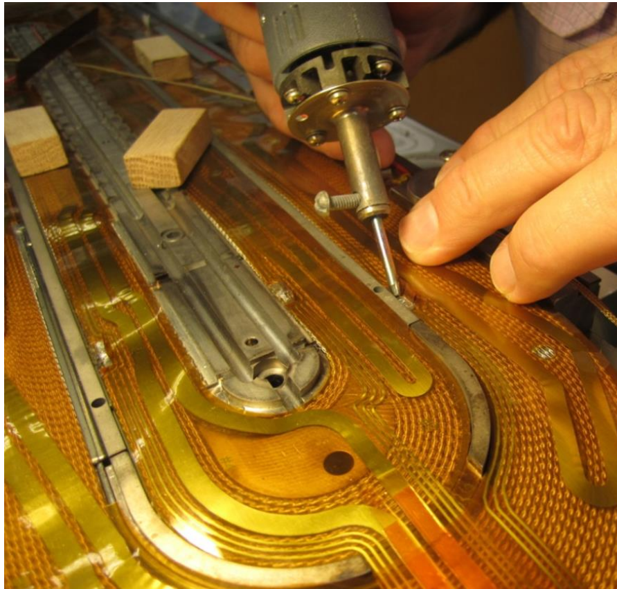
Figure 29: Voltage Tap and Quench Protection Heater Installation
