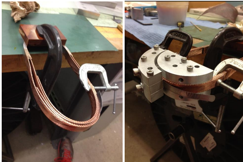
Figure 133: Applying Solder Between Cables
