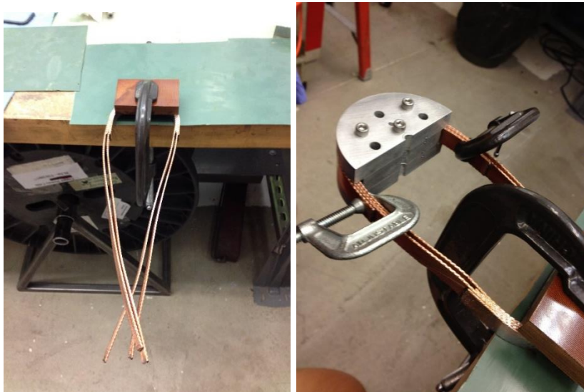
Figure 132: Pre-Bending Inter-Coil Joint
