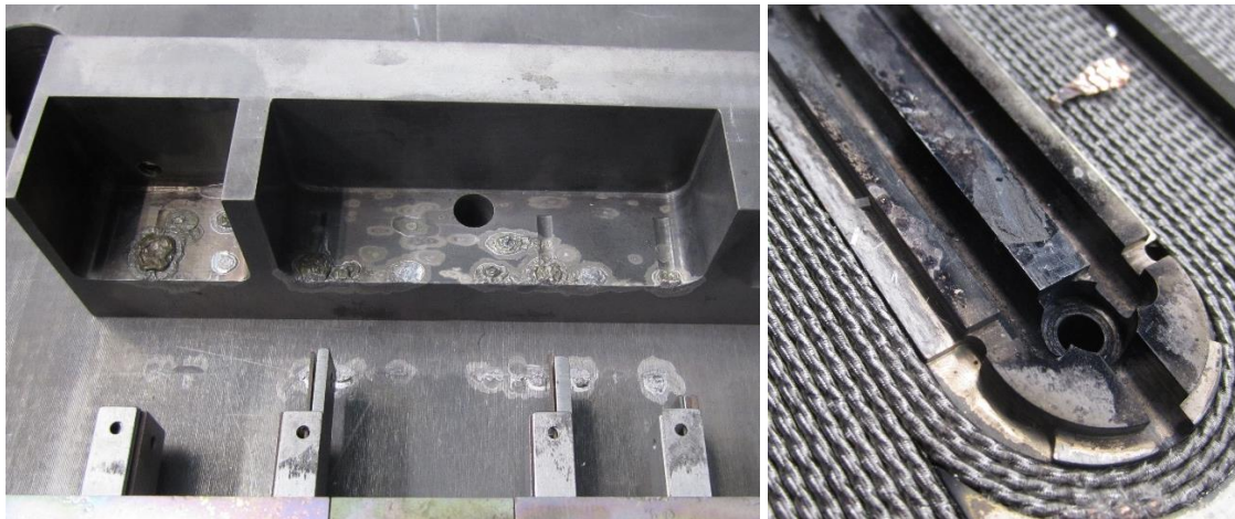
Figure 63: Location of Leaked Tin and Carbon Soot
