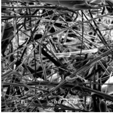
Figure 1.1: Microstructure and Macrostructure of glass wool (cf. [55])
