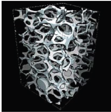
Figure 1.2: Microstructure of industrial foams (cf. [55])
