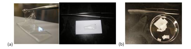
Figure 3.4: (a)Free-standing film of  $(LPEI_{8.5}/EMAA_{0.5wt\%})_{25}$ ; (b)free-standing film made without the first heating procedure.
