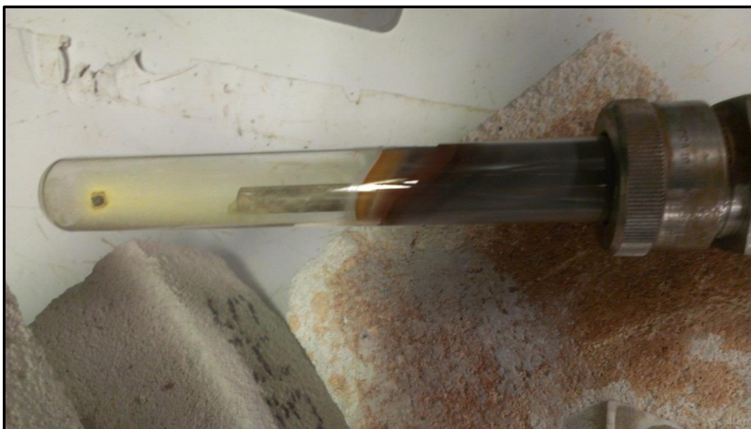
Figure 20: Reaction vessel as removed from heated block. Sample is U-50Zr from experiment UT-3.
