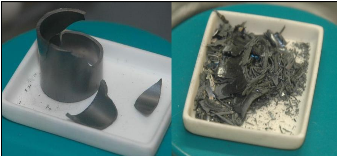
Figure 1: Comparison of hydride formation along the \beta -path (left) and \alpha -path (right). The sample on the left was produced at 582 °C with a hydrogen pickup of 90%. The sample on the right was produced at 432 °C with a hydrogen pickup of 86% [15].
