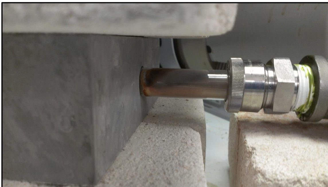
Figure 15: Reaction vessel containing U-50Zr (UT-2) in heated aluminum block; discoloration from suspended vapor deposited chloride solids.
