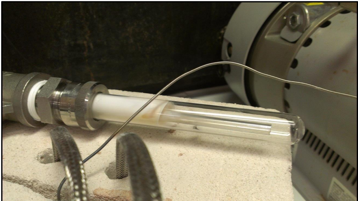
Figure 18: Reaction vessel from experiment UT-2 showing the white product on the cold zone wall; the Zr sample was completely gone.
