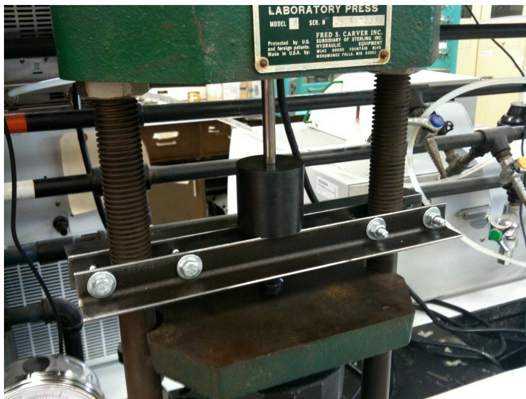
Figure J.8 Close-up of the punch and die system on the press just prior to compaction.
