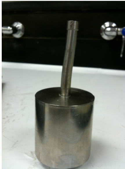
Figure K.1 Preliminary punch and die system with the longer punch bent.
