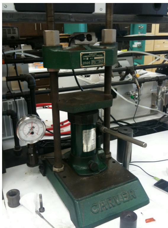
Figure J.3 Carver C Hydraulic Press in the Fuel Cycle and Materials Lab.
