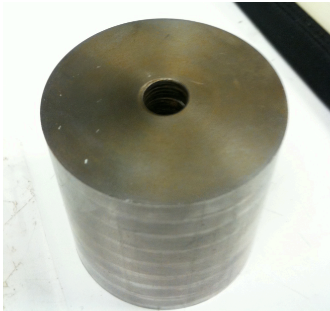
Figure K.3 Picture of the damage done to the lip of the die from the angular movement of the punch.
