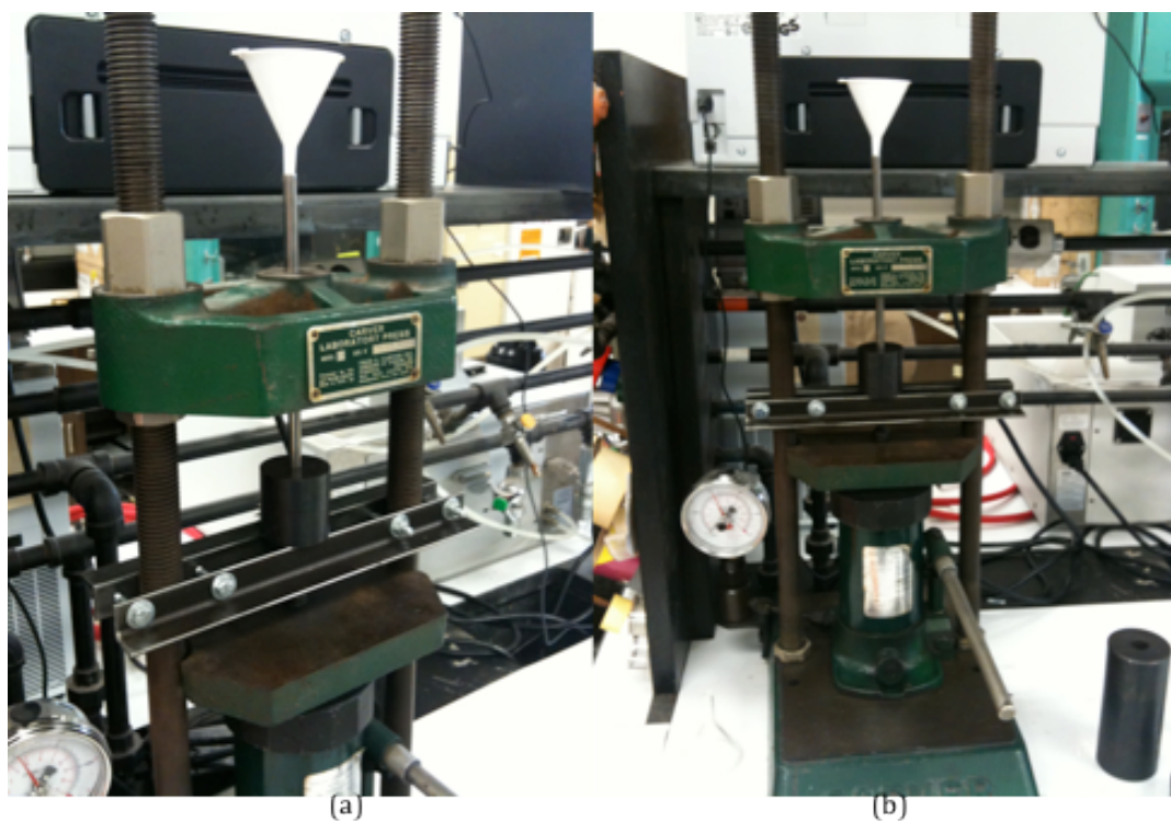
Figure J.9 Pellet pressing apparatus while filling the die with powder at two angles.
