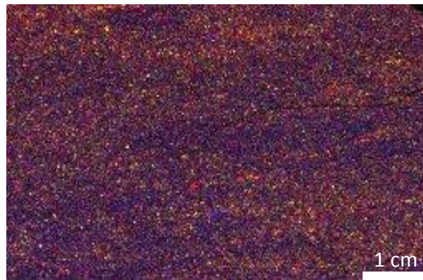
Figure 8. Moderately mineralized shale. Fase color compositional image with red = Fe K_{\alpha 1} fluorescence; green = S K_{\alpha 1} fluorescence; blue = Ca K_{\alpha 1} fluorescence.
