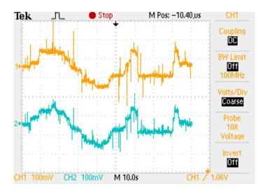
Fig. 2.12: Reference tracking performance of the power balancer circuit. Ch 2 is the current reference, the difference in source currents and Ch 1 shows the actual inductor current (1 div = 5A)
