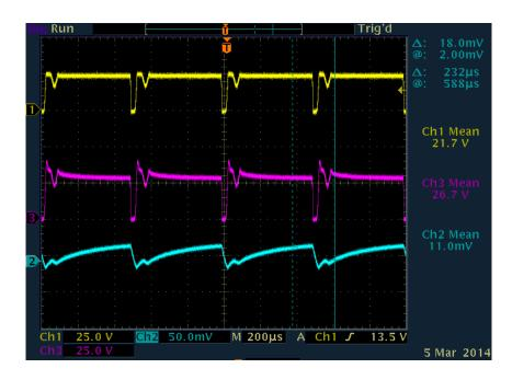
Fig. 4.22: Charging operation (buck) device voltages S<sub>3</sub> (Ch 1) and S<sub>4</sub> (Ch 3), and battery charging current (Ch 2)
