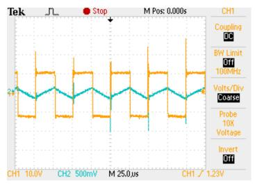
Fig. 2.11: Power balancing inductor voltage (Ch 1: 1 div = 10V) and current (Ch 2: 1div = 5A) waveforms under steady state operation. Inductor carries the difference between currents through the two sources.
