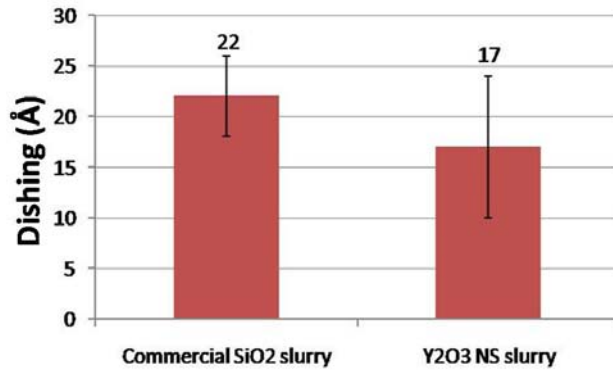
Figure 5.13. The Cu dishing in wafers that are polished using different slurries.
