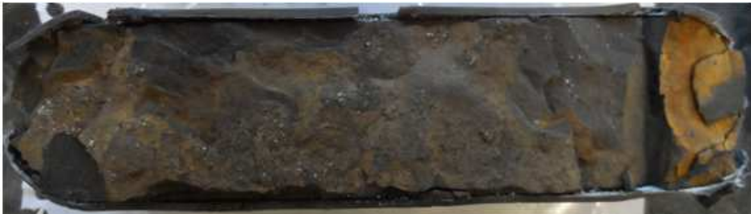
Figure 21 - FL2 fracture surface
