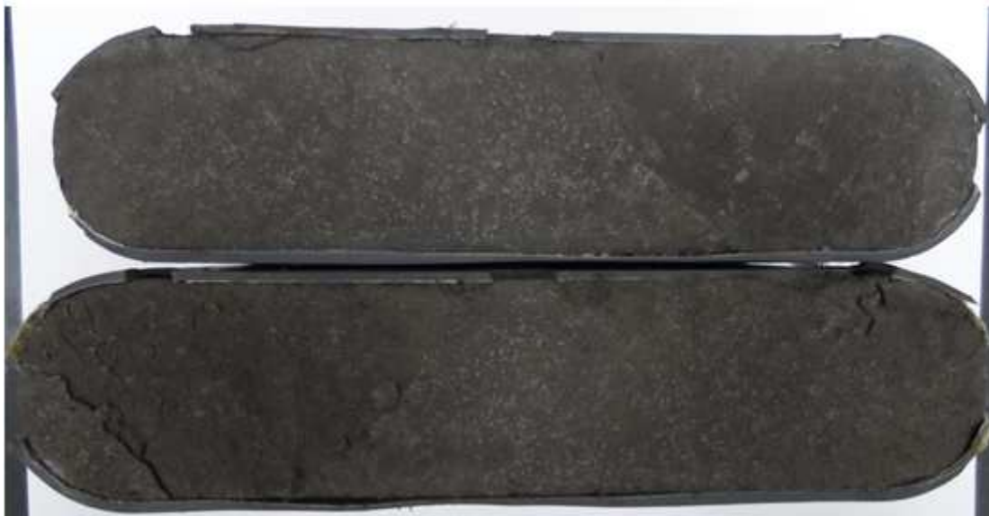
Figure 12 - Unpropped FL3 sample
