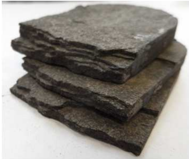
Figure 38 - FL3 crushed sample
