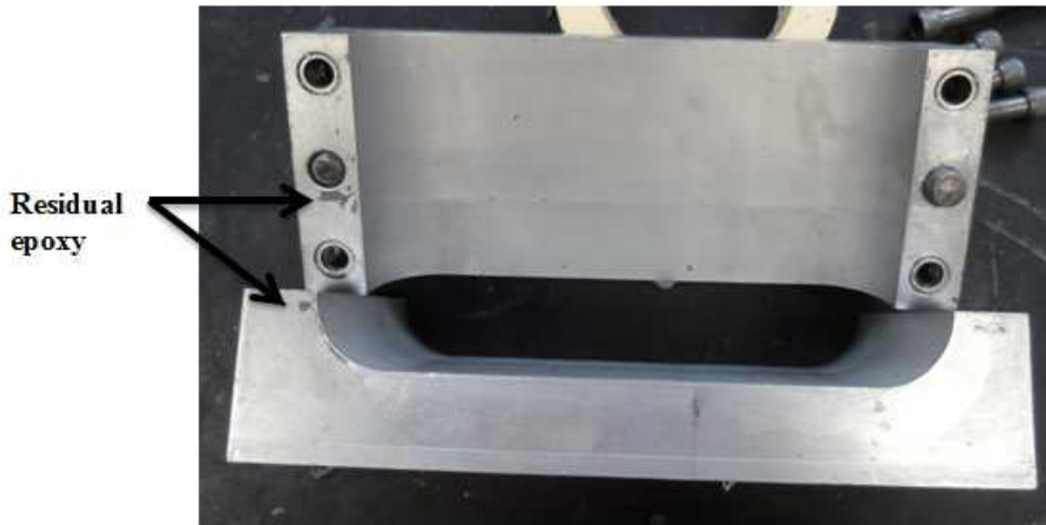
Figure 10 - Aluminum mold used for coating samples in silicone-base sealant
