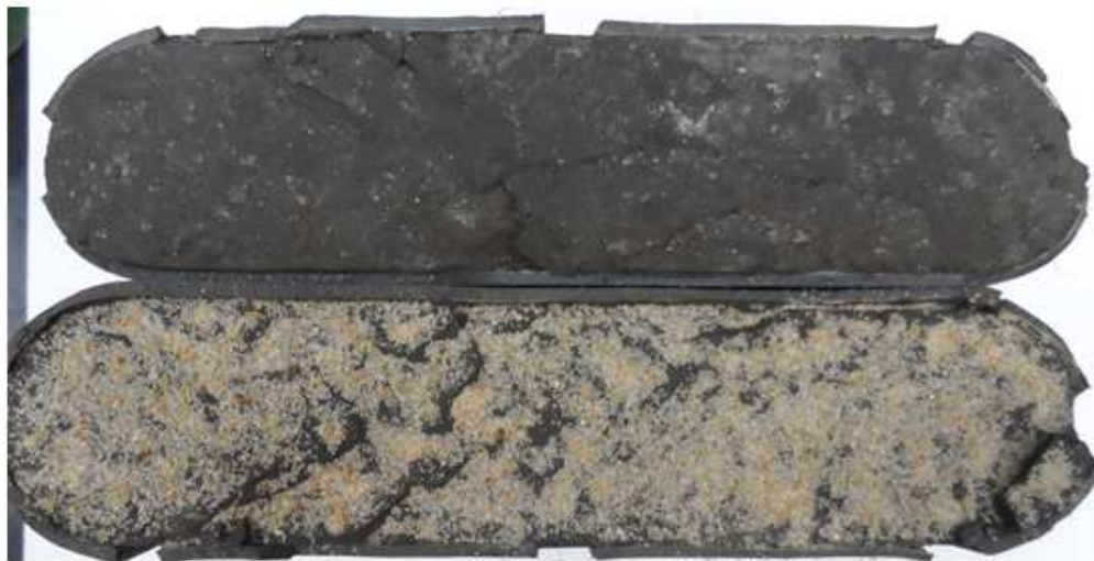
Figure 14 – FL3 sample with 0.1 lb/ft 2 30/70 mesh proppant before experiment
