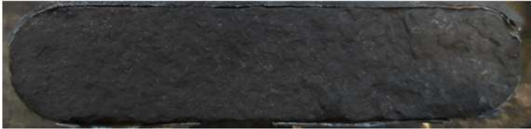
Figure 20 - FL3 fracture surface
