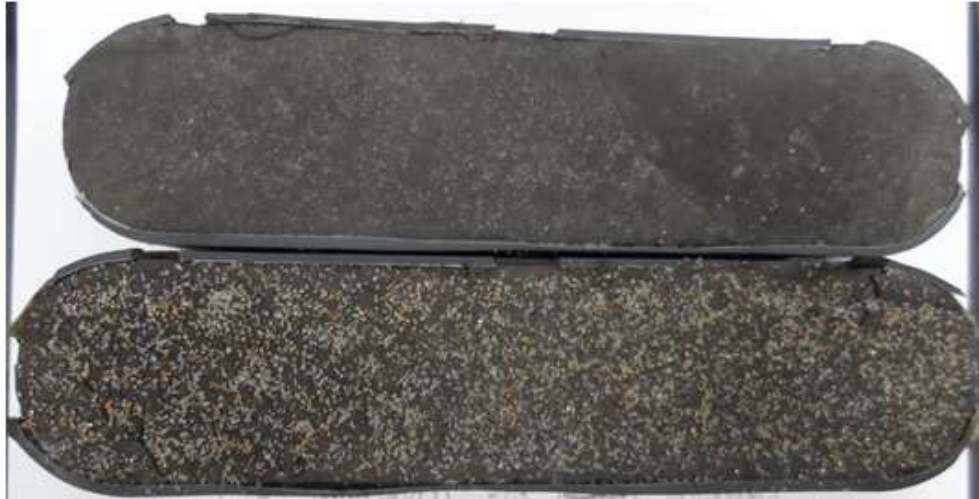
Figure 13 – FL3 sample with 0.03 lb/ft 2 30/70 mesh proppant before experiment
