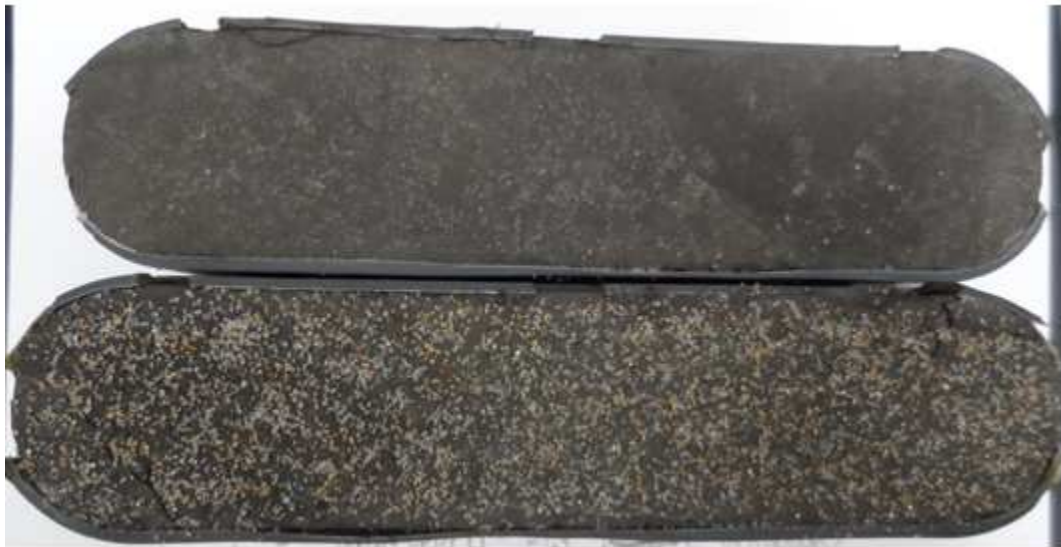
Figure 30 - low concentration proppant distribution on a FL3 sample
