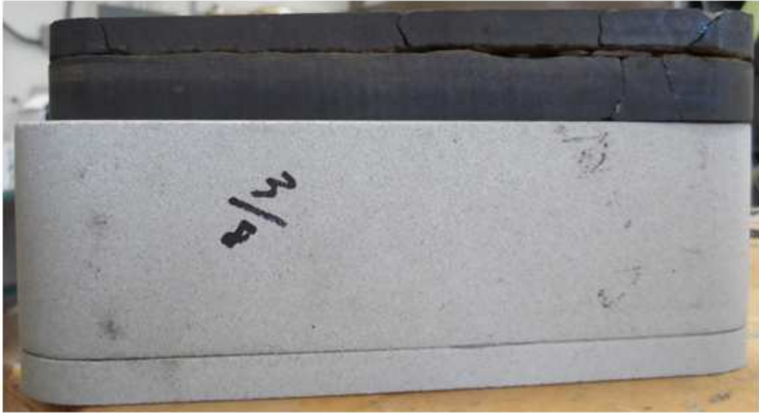
Figure 8 - Shale sample with sandstone cut to height allowing fracture centralization
