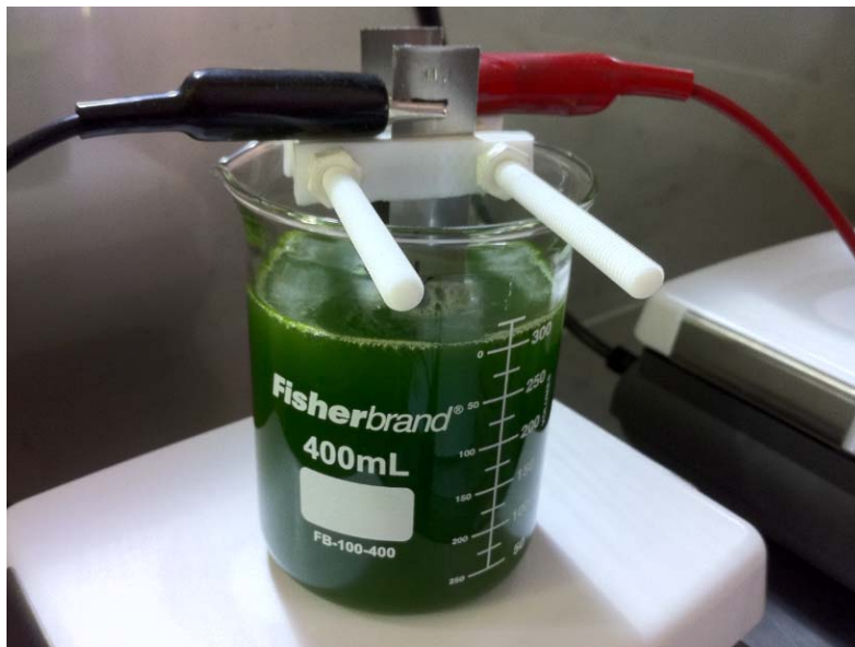
Figure 4: Electrocoagulation Experimental Apparatus - Including Electrical Connections, Electrodes, Electrode Holder, and Electrolytic Cell Containing Microalgae
