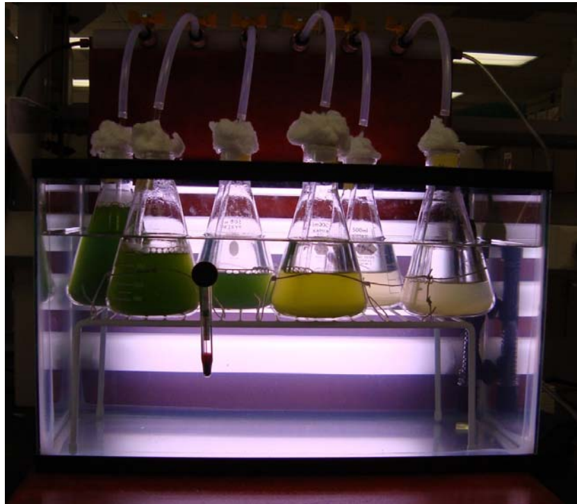
Figure 2: Cultures of Nannochloris oculata at Various Concentrations in a Temperature Controlled Water Bath and Fluorescent Lights
