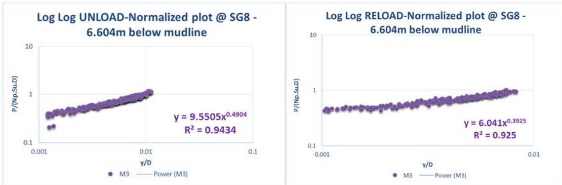
Fig. C-18: Power Law Fit To the Steady State Region of the Unload and Reload Loop of SG 8, for Motion M3
