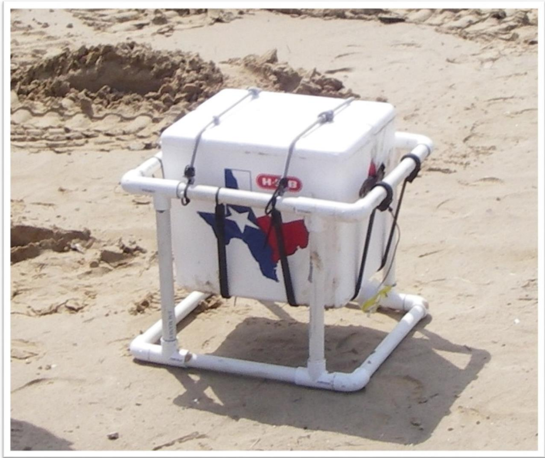
Figure 2.9. Polystyrene foam egg incubation container secured in PVC transport carrier with external temperature probe wire visible on right side. (Photo by Sharla Knoll.)
