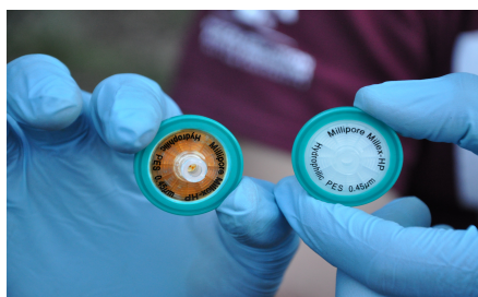
Figure 10. Comparison of a clean and used filter. A) Filtered versus clean B) There is a substantial amount of dissolved solids (orange) after a sample is filtered
