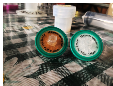
Figure 10. Comparison of a clean and used filter. A) Filtered versus clean B) There is a substantial amount of dissolved solids (orange) after a sample is filtered
