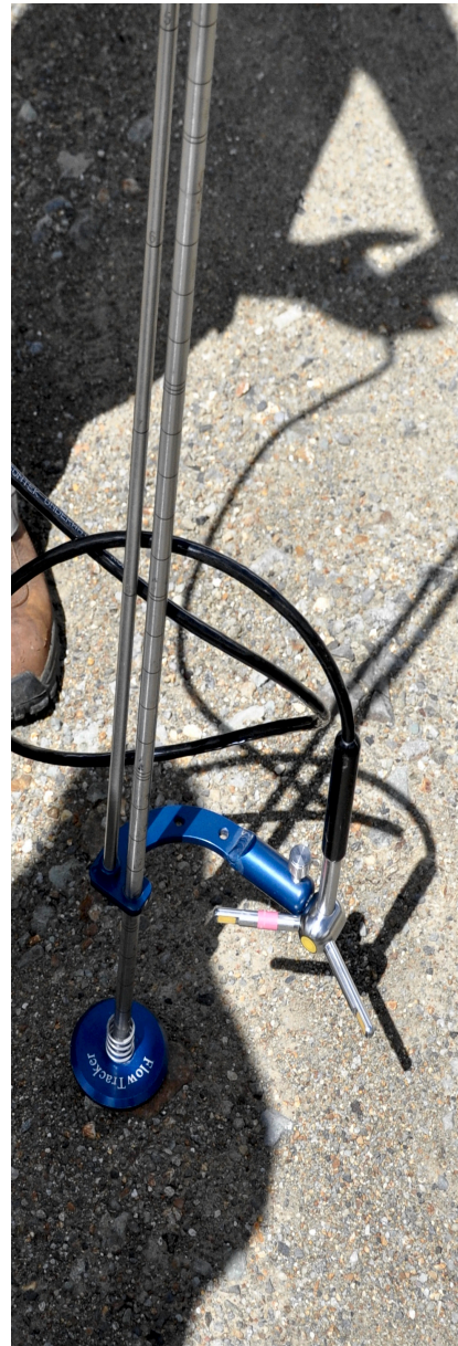
Figure 8. Photos of the Sontek/YSI FlowTracker Handheld Acoustic Velocimeter (ADV) with measuring rod. A) Equipment as a whole. B) Close-up of the 2 prong ADV
