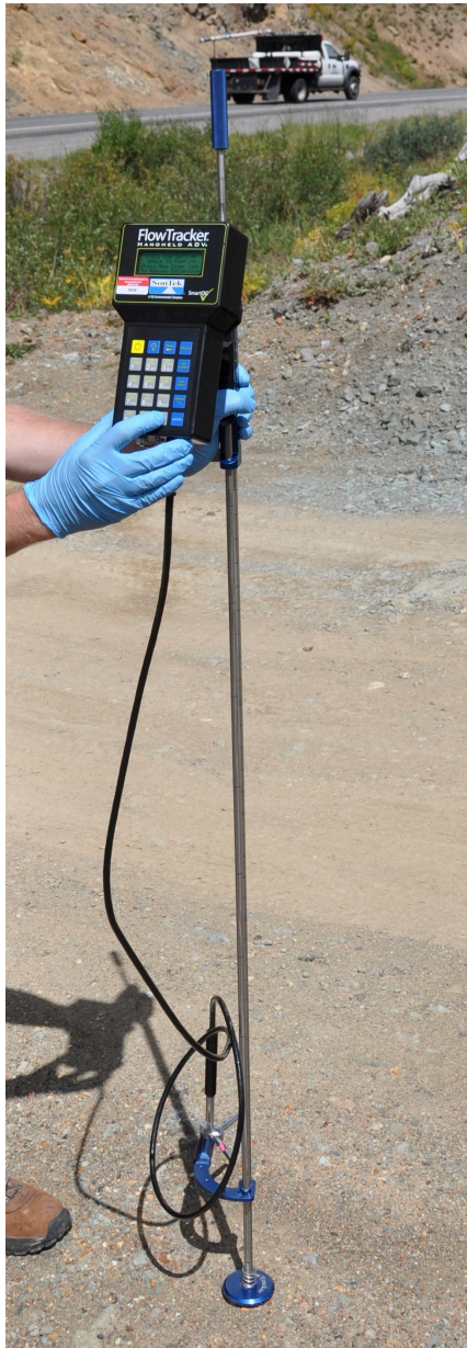
Figure 8. Photos of the Sontek/YSI FlowTracker Handheld Acoustic Velocimeter (ADV) with measuring rod. A) Equipment as a whole. B) Close-up of the 2 prong ADV
