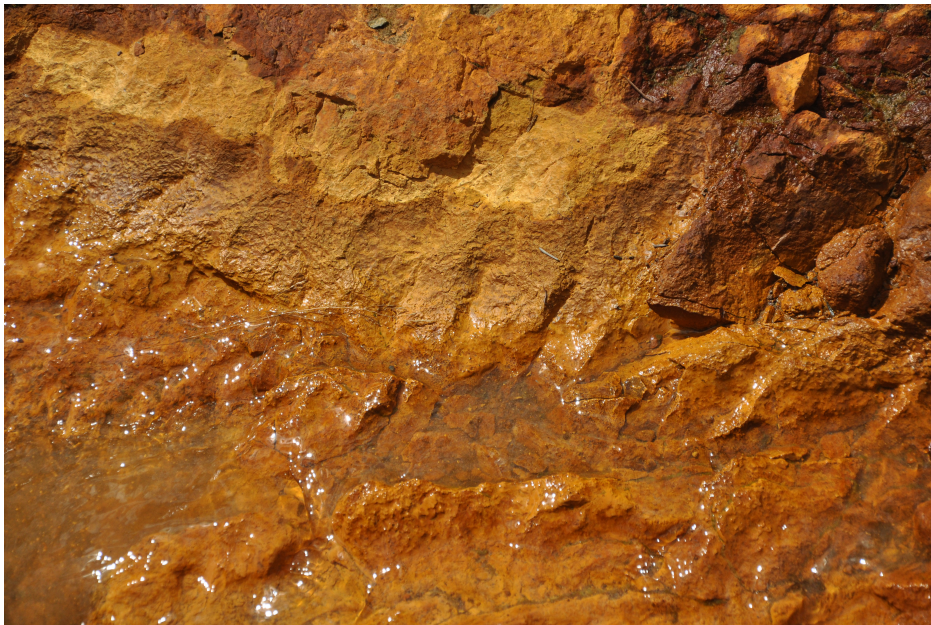
Figure 14. Orange iron oxyhydroxide precipitate from the mixing of RMC with the, Buried Tailings Seep. The low pH mixing with high pH causes iron to precipitate out
