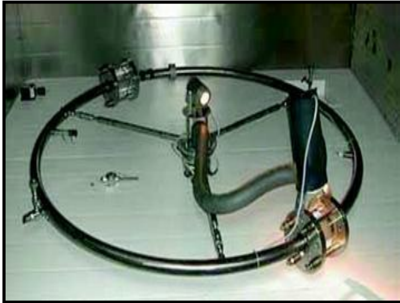
Figure 19: A wheel-shaped flow loop technique (laboratory scale) [57].
