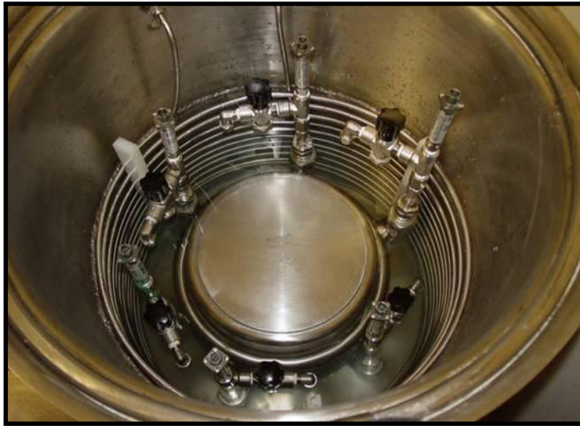
Figure 18: Mini flow loop technique from inside (laboratory scale) [57].
