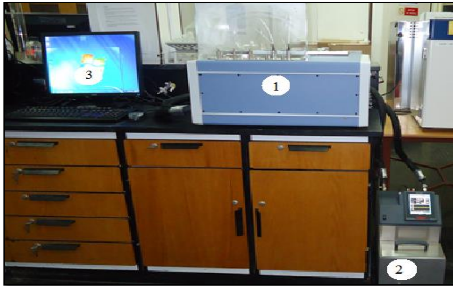
Figure 26: RC-5 experiment set-up are 1) base unit, 2) thermostat, 3) control-PC.
