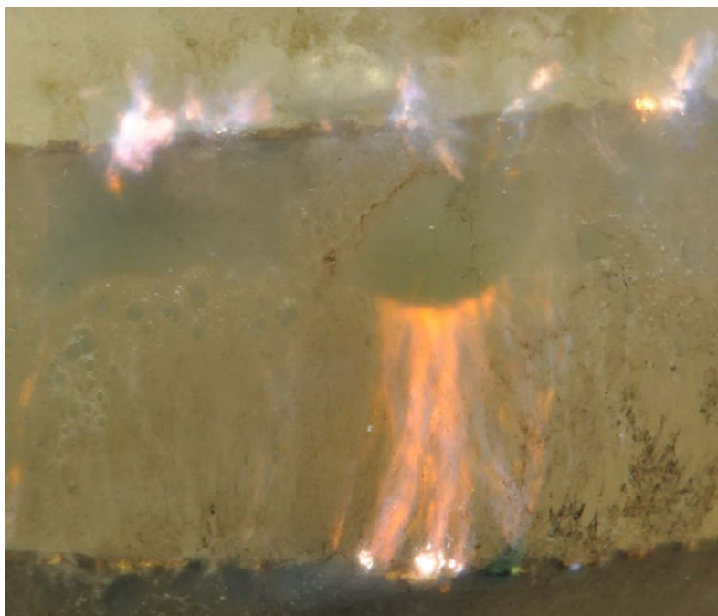
Figure 4 Plasma discharge in water and mineral oil mixture.
