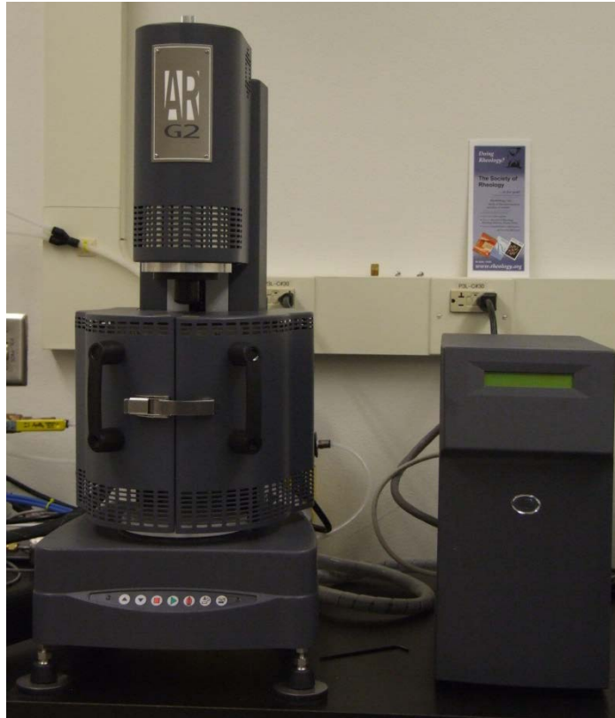
Figure 21 Picture of AR-G2 Rheometer used for viscosity measurements of heavy oils [40]
