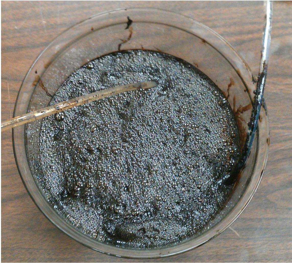
Figure 40 Oil mixture post-processing run with gas bubbling out of the processed mixture
