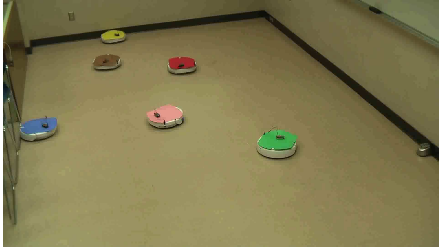
Figure 9.11: Experimental setup consisting of 6 iRobot Creates equipped with Epic motes.
