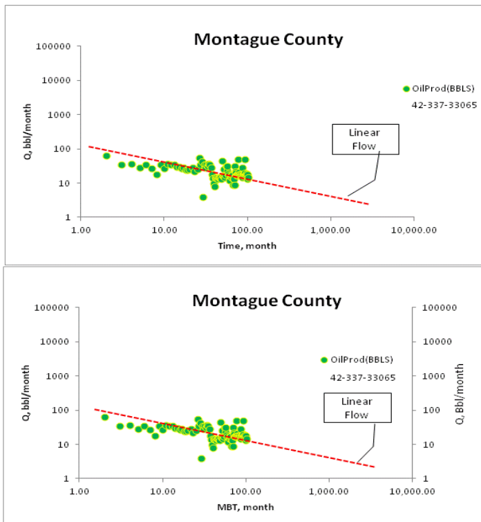
Fig. 63— Linear flow is the dominant regime for oil well API #33065 in Montague County, TX
