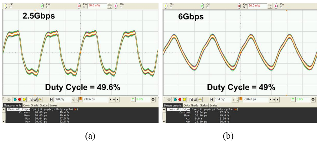
Fig. 4.23. Measured clock patterns ( 1010...) (a) at 2.5 Gbps and (b) at 6 Gb/s.
