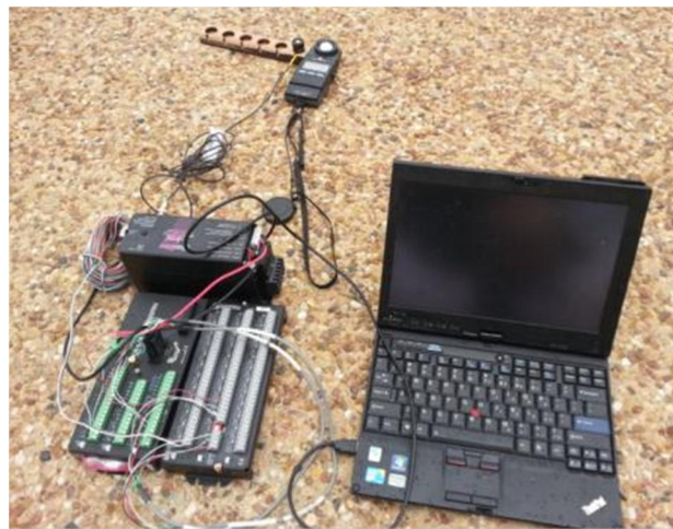
Figure B.1. Connections of the datalogger, sensors, and a laptop
