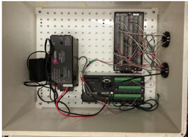
Figure B.4. Set up of datalogger with multiplexer
