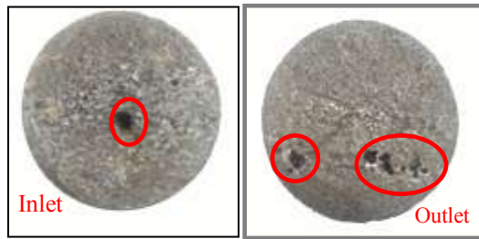
Fig. 37—Inlet and outlet face oil saturated cores at 5 cm 3 /min and 200°F.
