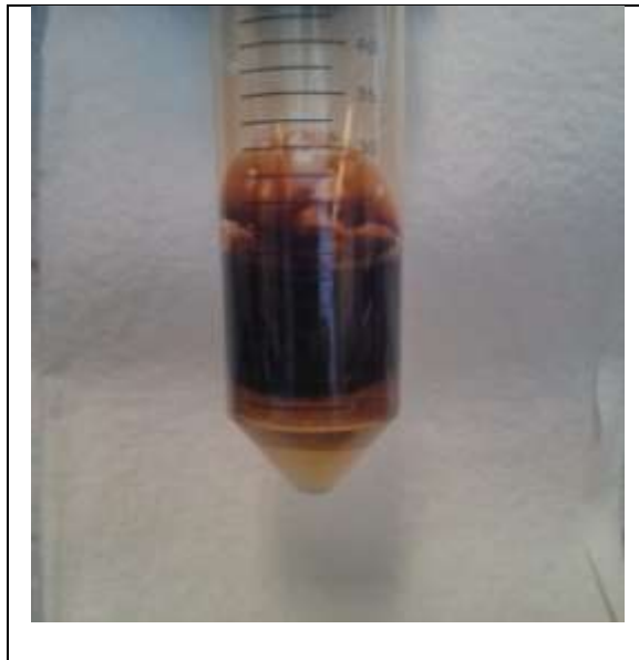
Fig. 1—Compatibility test between Naphthenic crude oil and HCl acid system
