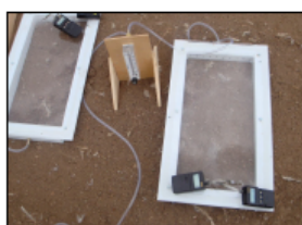
Odor characterization was performed by GC/MS analysis of volatiles collect by sorbent tubes from wind tunnel chambers placed on litter piles prior to land application.
