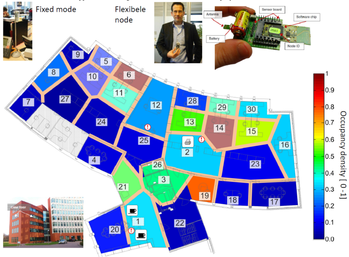
Figure 5. Floor plan with the measured grid in the case study office (orange), formed by 30 static nodes, Floor occupancy hotspots as factor of the most occupied spot during the measured period.
