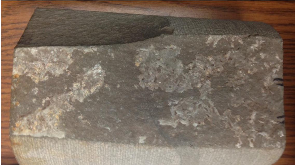
Fig. 38: Observed Mineralization On Fracture Surface From Spraberry Core
