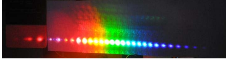
Figure 3.2: The photo of sidebands generated by PbWO_4 crystal recorded by a camera. These sidebands have been generated up to 23rd order in anti-Stokes side and at least 2nd order in Stokes side.
