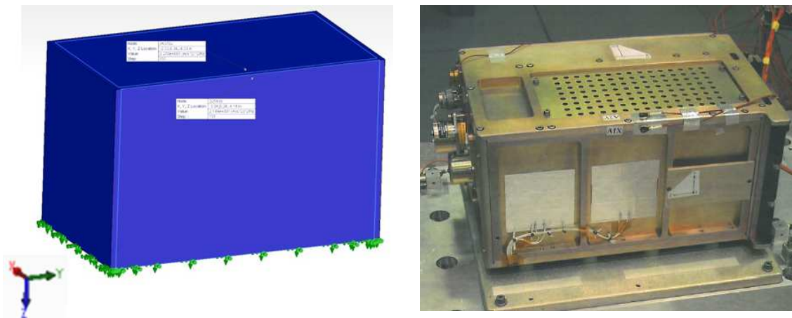
Figure 6.33. SSPL side PSD probe locations (left) and physical model with accelerometers (right)
