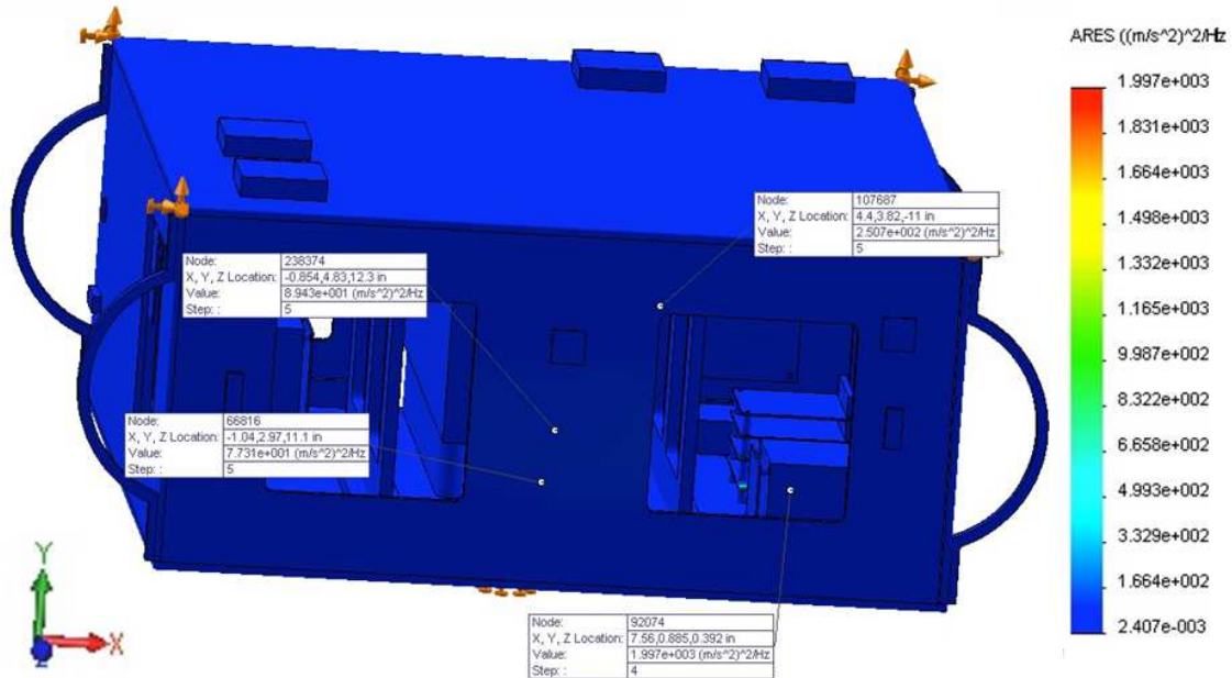
Figure 6.24. AGS4 PSD X-Axis probe locations
