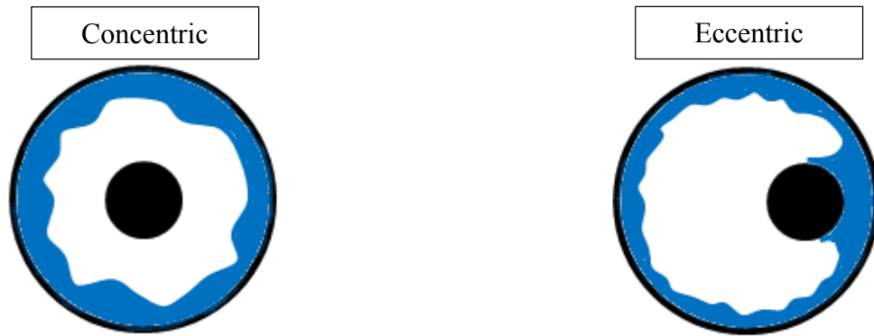
Figure 23: Liquid distribution around the annulus in concentric and eccentric positions.
