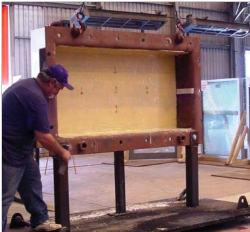
Figure C29. Hook crane to wall frame and unbolt frame from stand.
