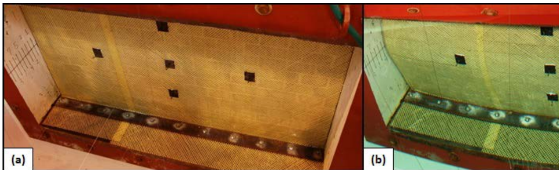
Figure 5.86. SW23. (a) Pretest view. (b) Deflection at 3 in.
