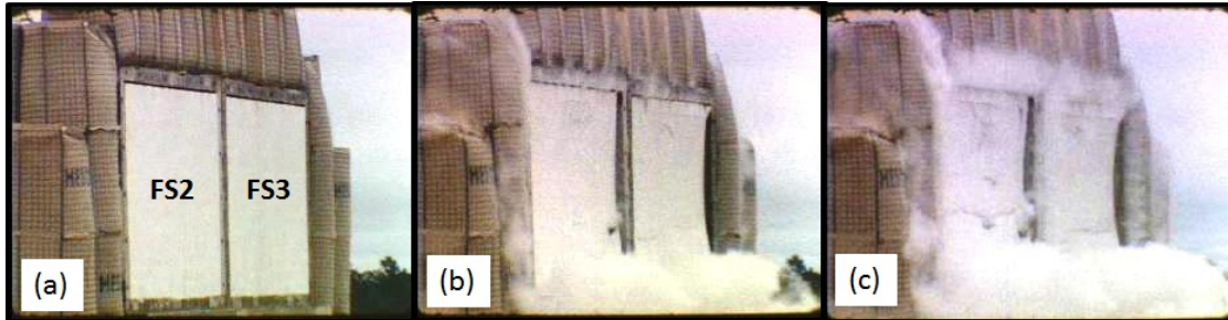
Figure 7.9. FS2 and FS3: High-speed video from exterior camera. (a) Pretest camera view. (b) Blast pressure impacts walls. (c) CMU blocks begin to disengage from retrofit.
