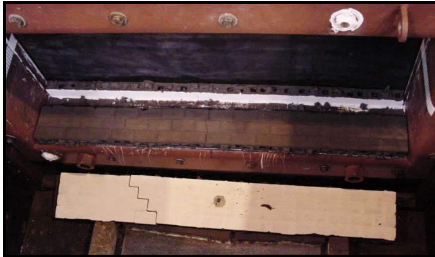
Figure 5.6. Posttest view of wall debris in chamber.
