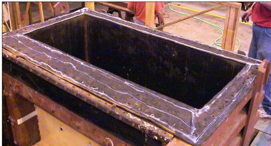
Figure C19. Apply another layer of silicone on neoprene seals before the lid is attached.
