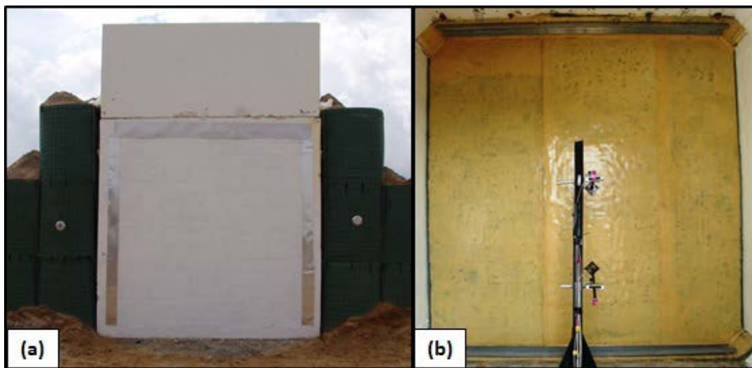
Figure 7.45. FS13. (a) Pretest exterior view with aluminum flashing covering the gaps. (b) Pretest interior view.
