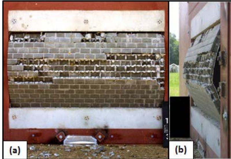
Figure 6.17. DW5. (a) Exterior view. (b) Permanent deflection.
