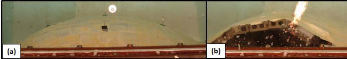
Figure 5.44. SW13. (a) Deformation extends past the reaction structure frame. (b) Failure of the film occurred when the material sheared at the top support.
