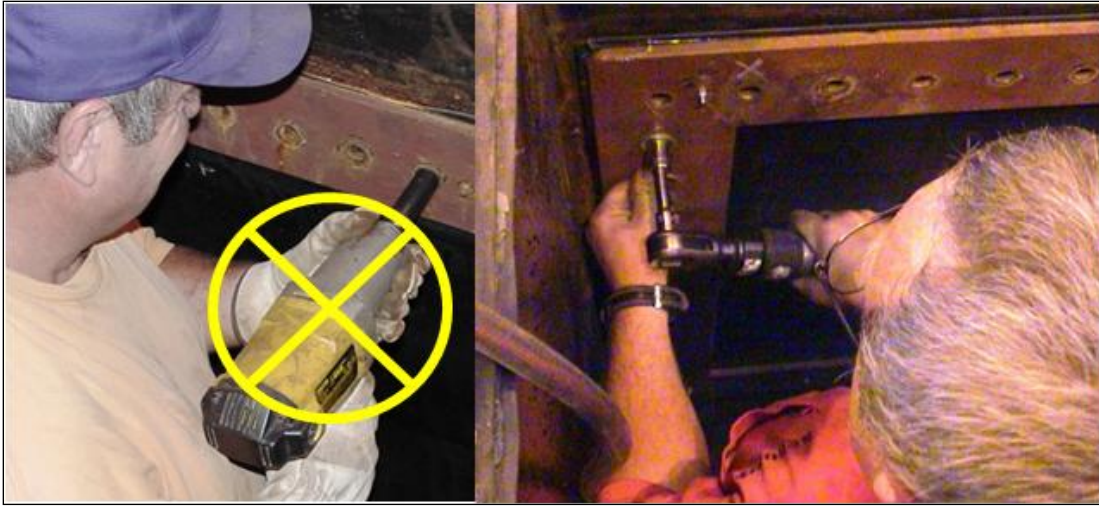
Figure C12. Bolt membrane steel frame to pressure cavity. Do not use an impact wrench; use an air or torque wrench.
