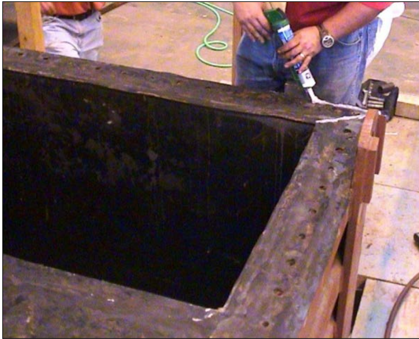
Figure C18. Apply silicone to steel edges of pressure vessel then apply neoprene seals.
