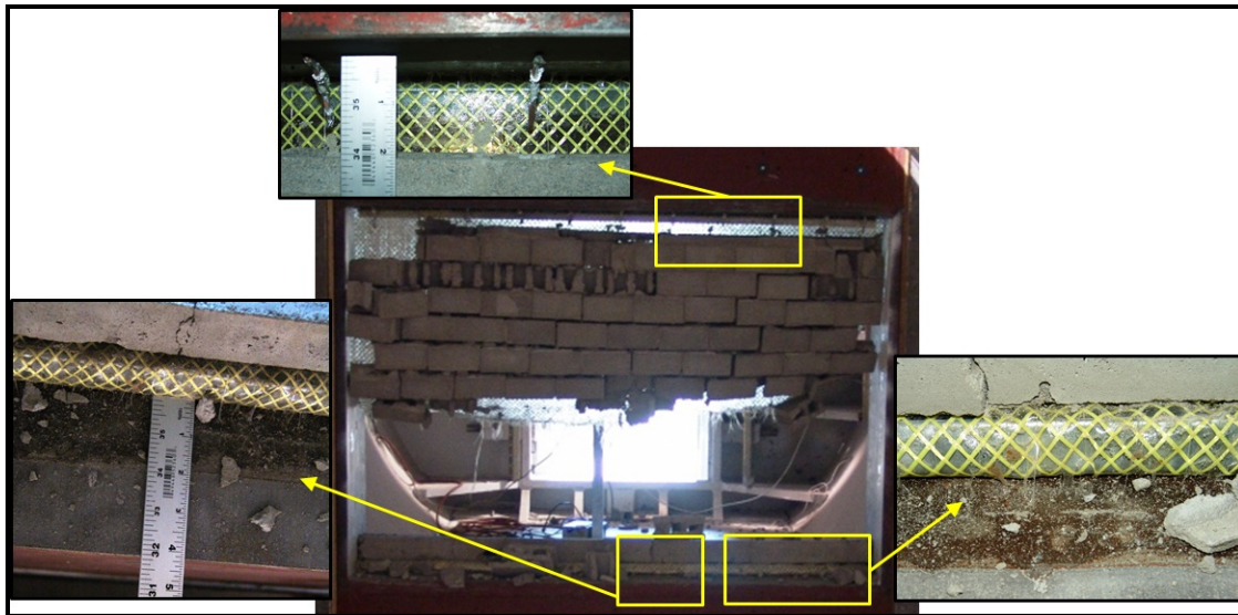
Figure 6.78. BLS9: Exterior view of anchor plates on the supports and damaged wall/retrofit materials. (Adapted from Johnson, Davis, Coltharp, Durst, and Smith 2010)
