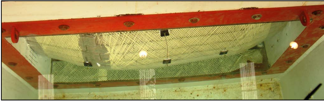
Figure 5.81. SW22 – maximum wall deformation transitioned from mid-height to the seam/overlap area. (Johnson, Davis, Coltharp, Durst, and Smith 2010)
