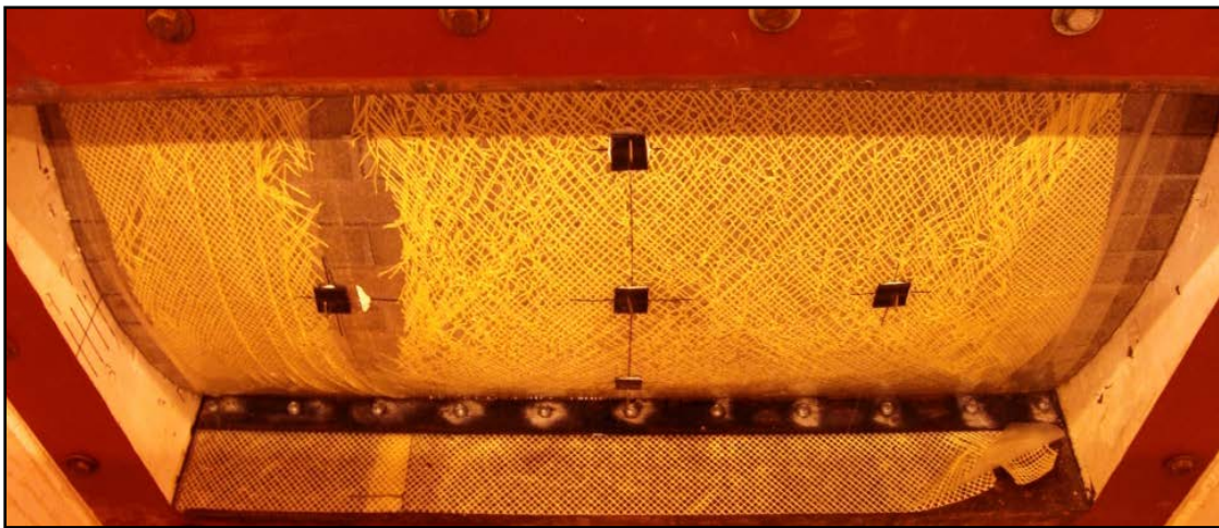
Figure 5.82. SW22 – Once pressure was relieved the fiber reinforcement was permanently deformed. (Johnson, Davis, Coltharp, Durst, and Smith 2010)
