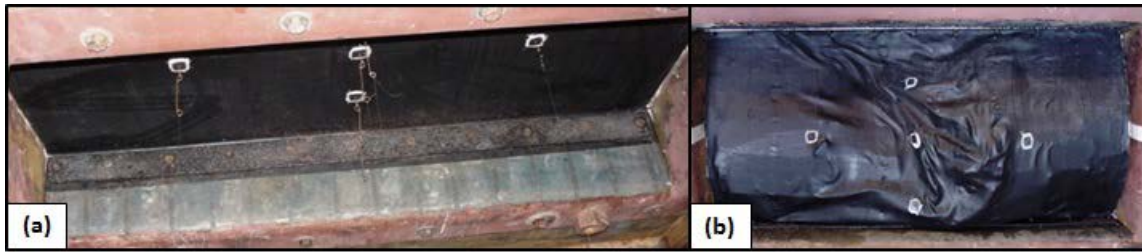
Figure 5.62. SW17. (a) Pretest view. (b) Posttest view of the retrofit system.
