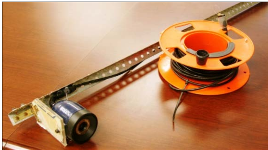
Figure C44. Underwater video camera.
