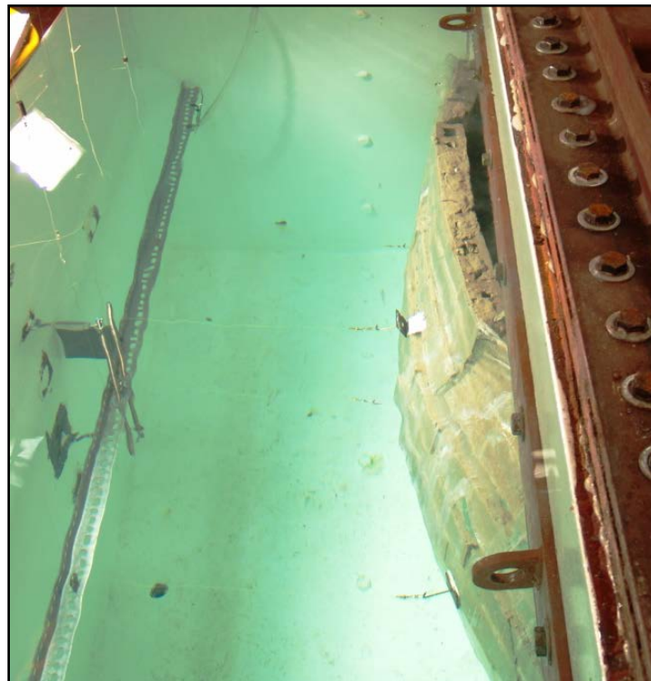
Figure 5.74. SW20– Final failure occurred as the film tore across the top support. (Johnson, Davis, Coltharp, Durst, and Smith 2010)
