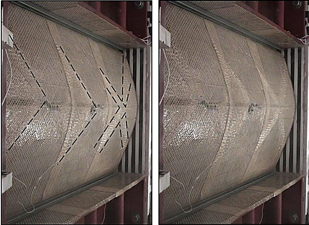
Figure 6.83. The two photos illustrate the pattern created in the elastomeric film at high stress and strain areas.
