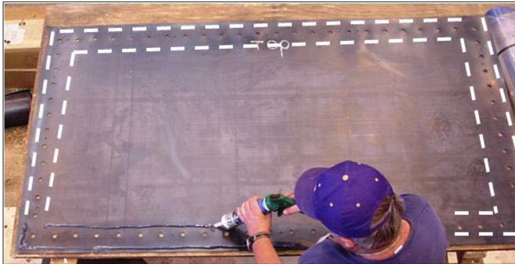
Figure C10. Apply two solid beads of silicone to membrane (one along perimeter and one just inside the bolt holes) before it is attached to pressure cavity.
