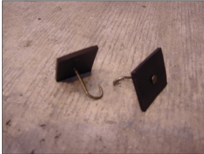
Figure C26. Deflection gauge mounts made from nails and neoprene squares.
