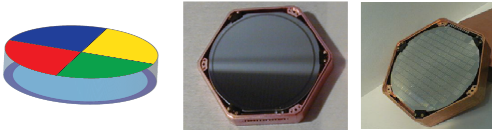
Figure 3.1: Left to right: Schematic of ZIP detector, with phonon sensors (4 independent phonon measurement channels arranged in quadrants) and charge sensors (2 concentric aluminum electrodes); A picture of fabricated charge electrodes (taken from [239]); A picture of fabricated phonon sensors (taken from [231]). The sections below discuss relevant details on corresponding signal generation and measurement.
