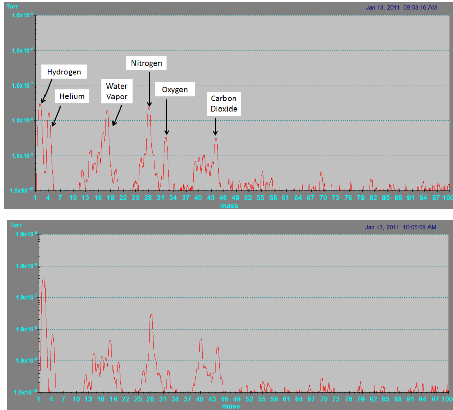
Figure 5.10: Comparison of gas levels in deposition chamber, before and after aluminum bury. A reduction in water vapor and oxygen levels is found, along with suppression of gases with heavy molecular mass (formed from the decomposition of pump oil vapors)
