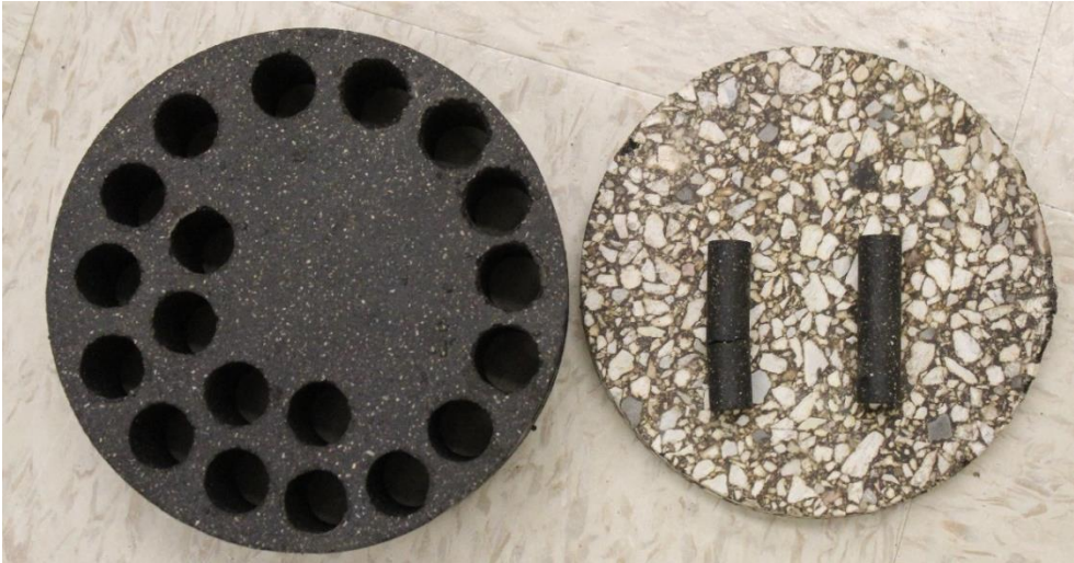
Figure 7. DMA Cylindrical Specimen
