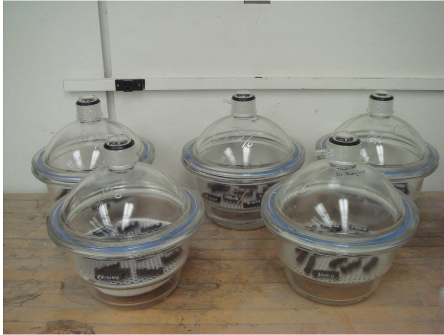
Figure 10. DMA Specimens Aging in Desiccators
