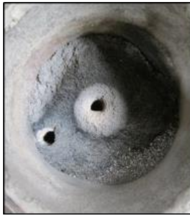
Figure 32. Air bypassing around the thermowell (from E4 postmortem)
