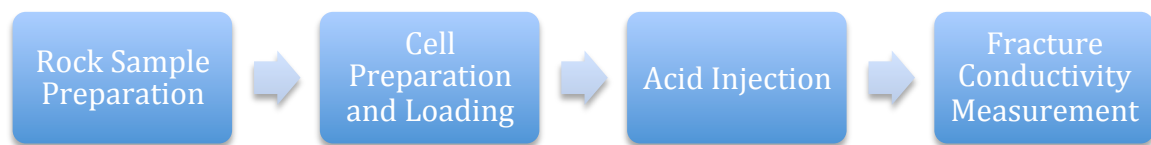
Figure 7: Experimental Procedure Flowchart
