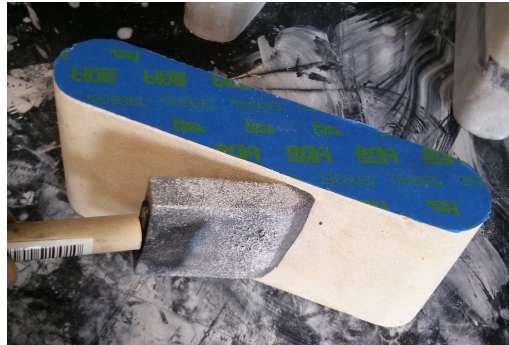
Figure 9: Application of Silicone Primer
