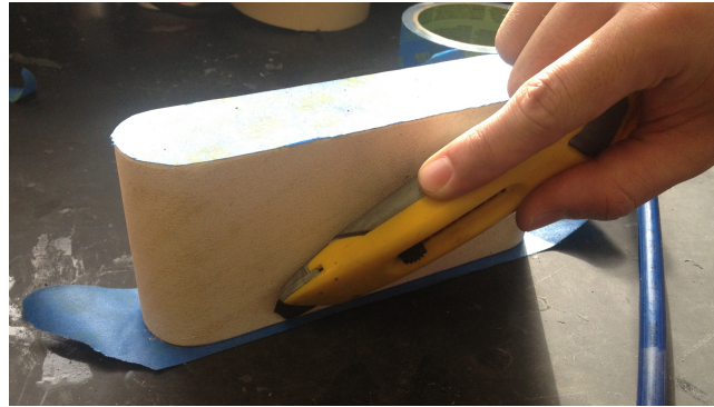
Figure 8: Example of Removing Excess Tape from Rock Sample
