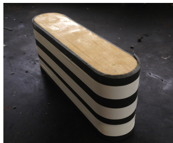
Figure 12: Placement of Teflon Tape on Rock Sample
