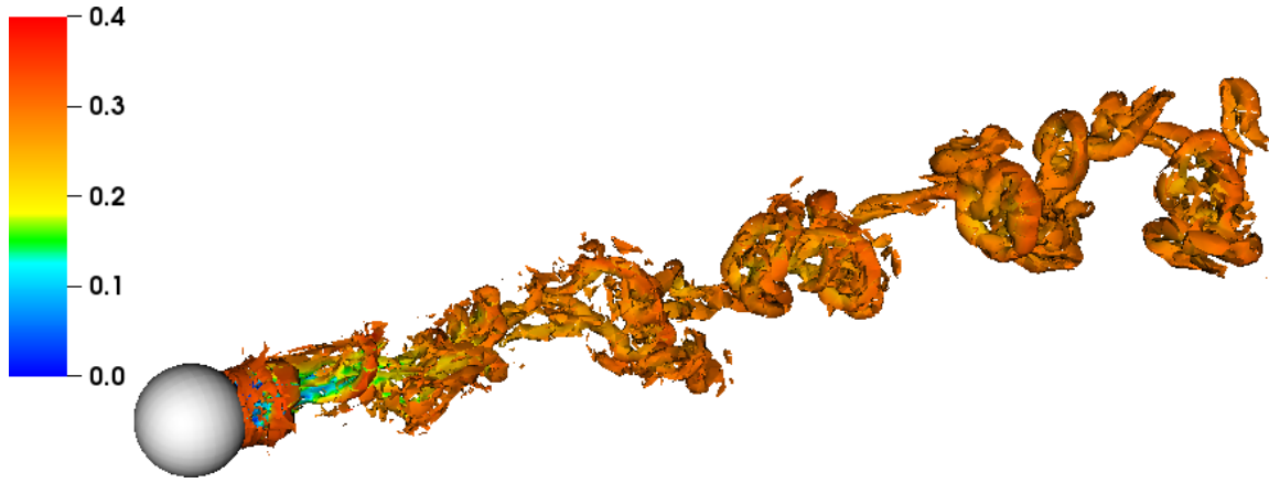
Figure 3.18: Small scale structures in subsonic sphere flow at Re = 1000 . Isosurfaces of \lambda_2 = -0.001 are shown, colored by Mach number.
