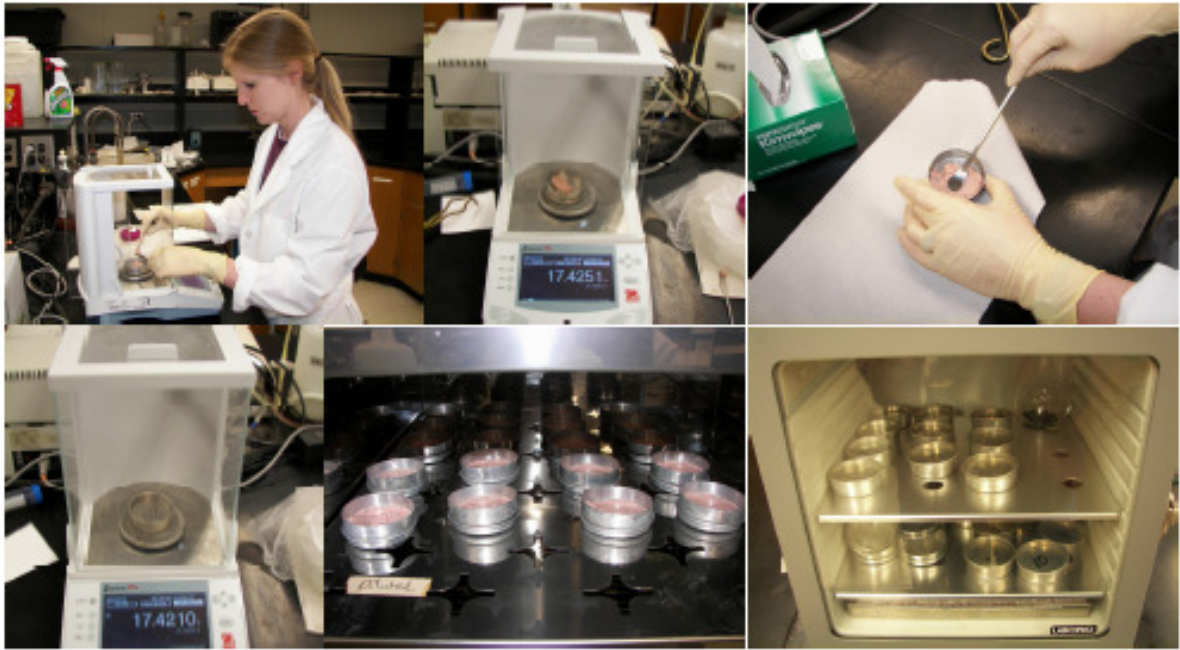
Figure A-2. Sample Preparation for Moisture Analysis Using the Oven Drying Method (AOAC 950.46).
