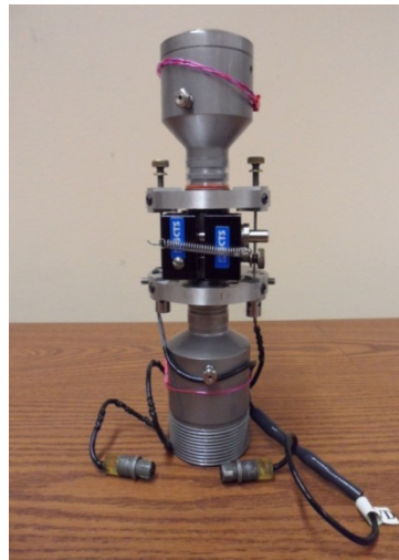
Fig. 3.1 Photo of rock specimen installed with loading platens and LVDT transducers
