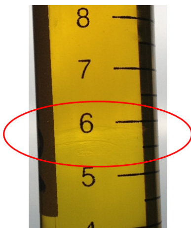
Fig. 13—Phase separation face in the sample of VES-1-based acid with 1,500 ppm Fe (III) at a HCl concentration of 20 wt% at room temperature.
