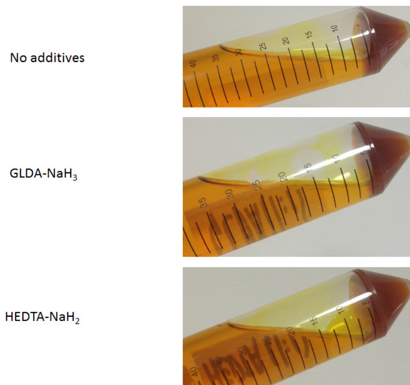
Fig. 29— VES-2-based acids: 4 vol% VES-2, 8,000 ppm Fe (III), and 20 wt% HCl.
