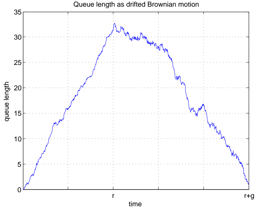
Figure 2.2: Illustration of queue length as Brownian motion in one cycle assuming r and g large enough. Brownian approximation allows the queue length occasionally to decrease a little during the red signal.
