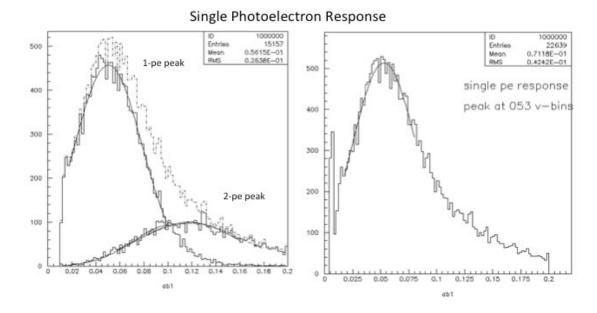
**Fig. 37.** Single photoelectron response from NaI(Tl) PMT. Left: Total low energy response divided into single and double photoelectron gaussian peaks. Right: Single photoelectron peak with a gaussian fit, mean value of 0.053 in area units for the PMT.
