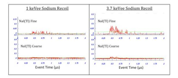
**Fig. 36.** Signals from a 1 keVee and 3.7 keVee nuclear recoil in the NaI(Tl) recorded with the Acqiris DC265 digitizer. Top: Fine scale NaI(Tl) channel. Bottom: Coarse scale NaI(Tl) channel.
