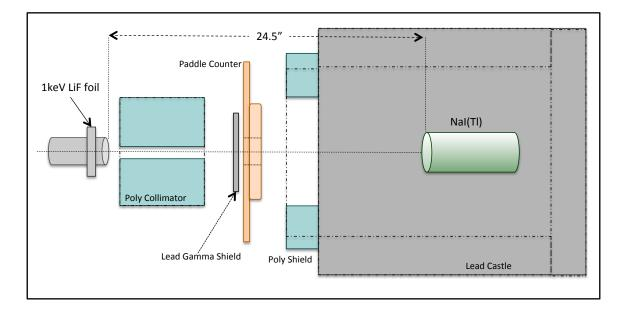
Fig. 29. Neutron scattering apparatus setup.
