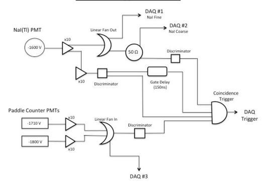
**Fig. 35.** Hardware trigger electronics chain for our experiment. Signals from the NaI(Tl) PMT and the paddle counter PMTs are amplified, split then sent to an input channel of the DAQ and through a discriminator. The discriminator signals are sent to the external trigger of the DAQ, which is set as a coincidence between the NaI(Tl) and the paddle or as a self coincidence in the NaI(Tl).
