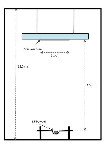
Fig. 31. Evaporation chamber for LiF coated stainless steel.
