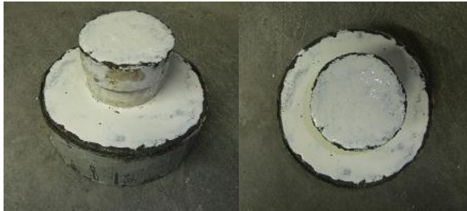
Figure 3-10 Curing compounds applied on dielectric constant measuring specimen
