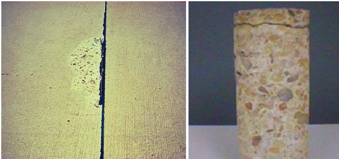
Figure 2-4 Spalling (left) and horizontal delamination [12, 15]
