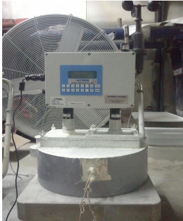
Figure 3-4 The ACMM system standing on a concrete specimen sprayed with curing compound
