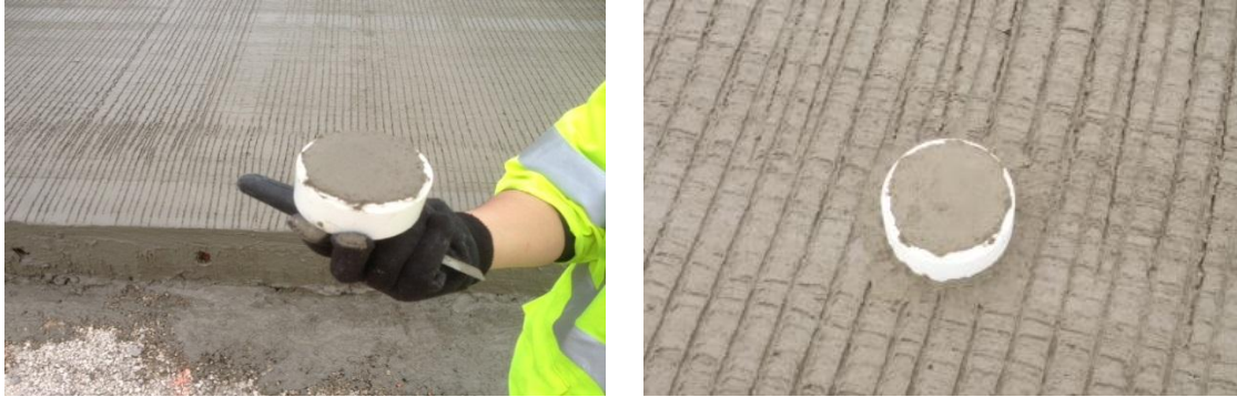
Figure 5-2 Cylindrical mold for DC measurements
