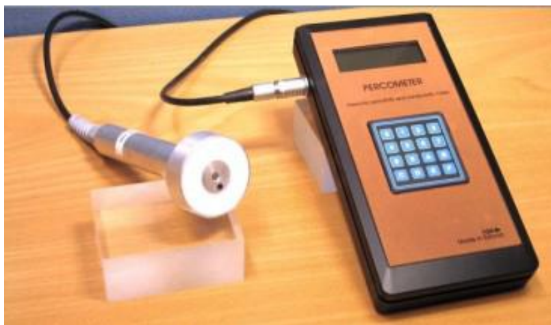
Figure 3-8 The Adek™ Percometer and the probe [51]
