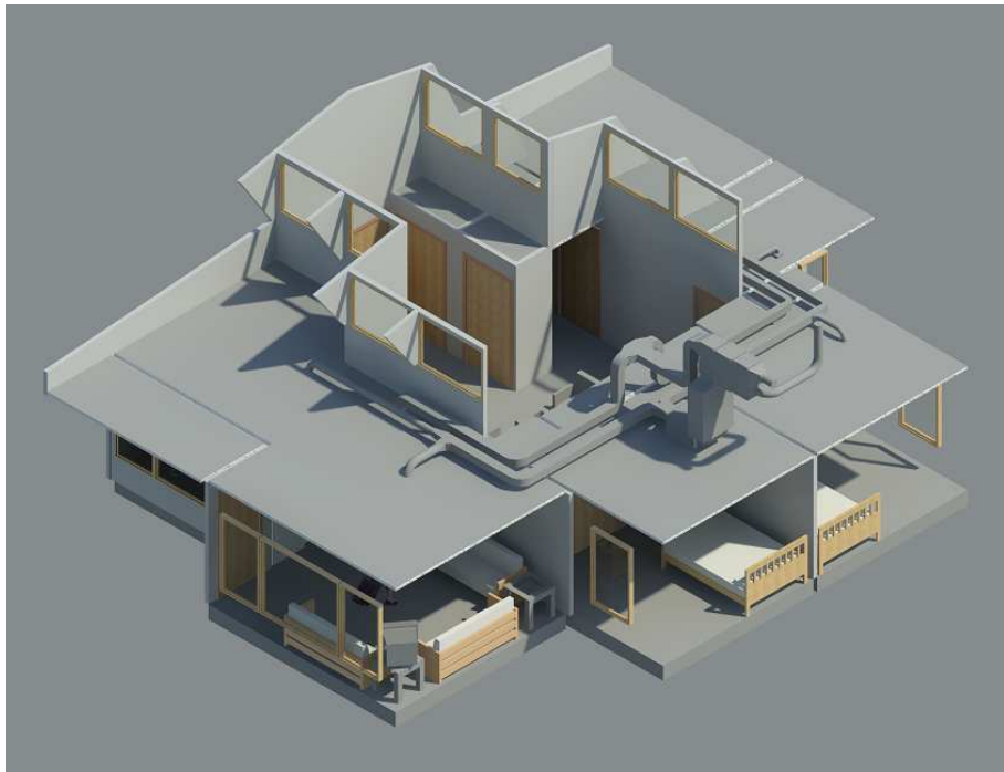
Figure 3.33: The 3-D southeast view of the duct layout of the atrium house with an outdoor air system before the implementation of the partial conditioning strategy.
