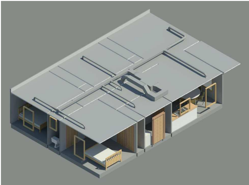
Figure 3.14: The air duct layout of the negatively pressurized, multizone baseline Habitat for Humanity house.
