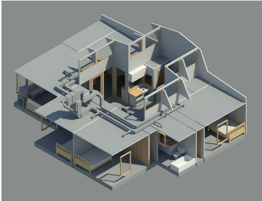
Figure 3.32: The 3-D northeast view of the duct layout of the atrium house with an outdoor air system before the implementation of the partial conditioning strategy.
