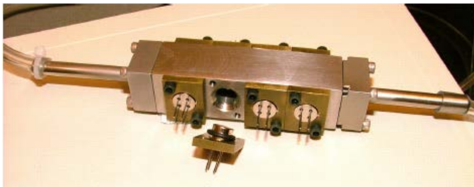
Figure 49 Close-up of the sensor chamber. This view displays four MOX sensors mounted on one side of the chamber. The other side contains three other MOX sensors and a temperature/humidity sensor.
