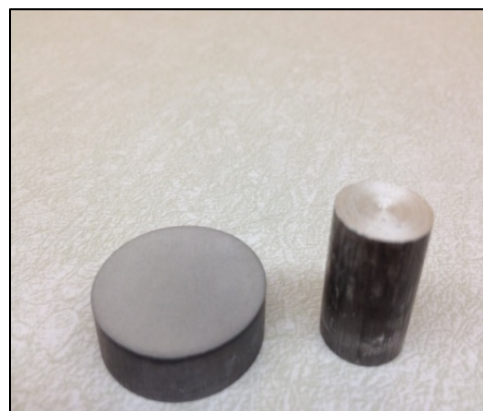
Figure.2.1. Sintered Al-Al 2 O 3 composite samples of diameters 25.4 mm and 12.7 mm respectively
