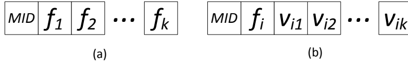
Figure 5.12: Multicast packet format: (a) output packet to the requested node; (b) output packet to a facility node.
