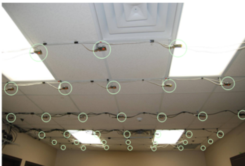
Figure 5.2: Our testbed with 42 TelosB motes.
